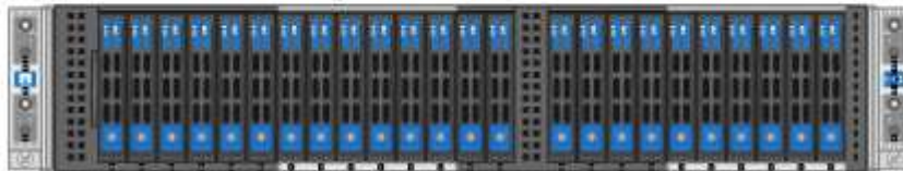
H410S storage nodes in a four-node chassis
