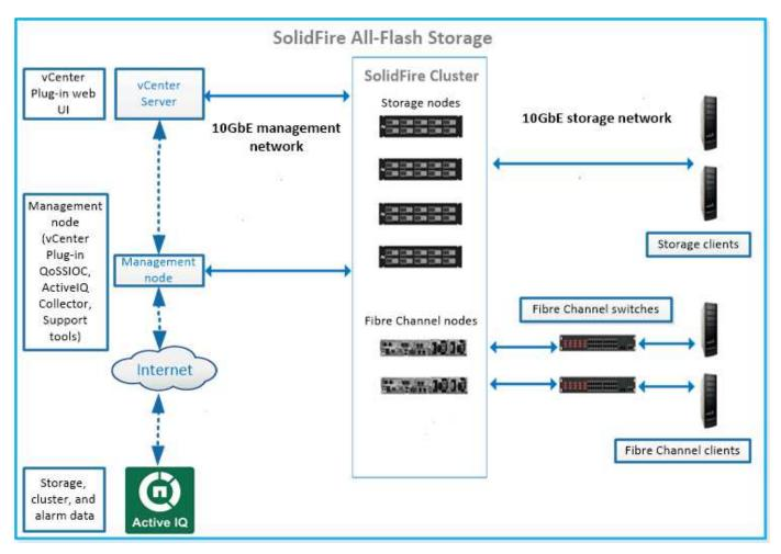
You can manage, monitor, and update the system using the Element web UI and other compatible tools:
