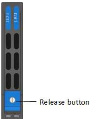
When you press the release button, the cam handle on the drive springs open partially, and the drive releases from the midplane.
