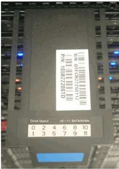
2. Verify that the serial number on the service tag matches the NetApp Support case number when you ordered the replacement chassis.
