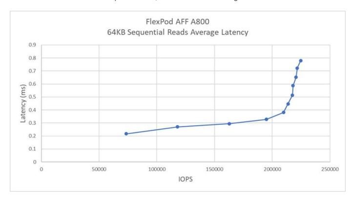
In our testing, we found that the system achieved around 250k IOPS while maintaining just under 1ms of server-side latency.
