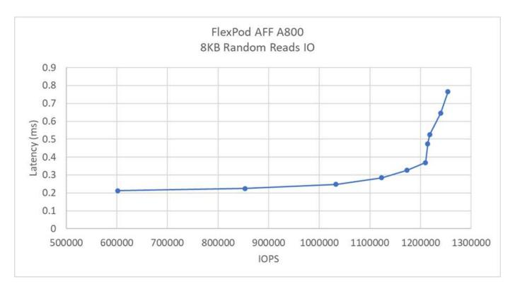
In our testing, we found that the system achieved over 1.2M IOPS while maintaining just under 0.35ms of server-side latency.
