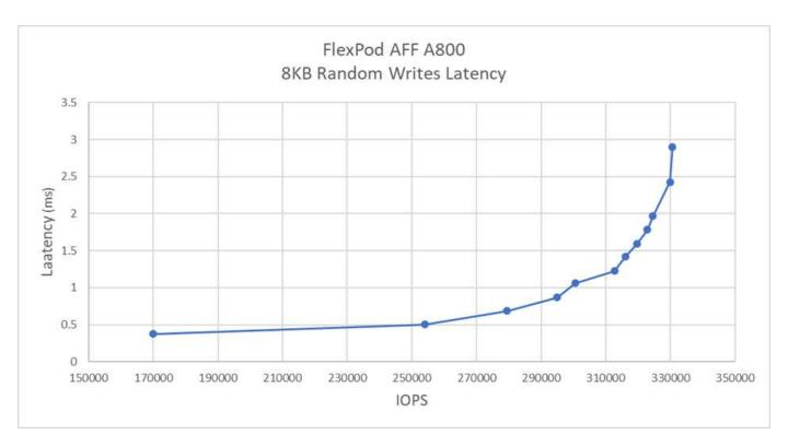
In our testing, we found that the system achieved close to 300k IOPS while maintaining just under 1ms of server-side latency.
