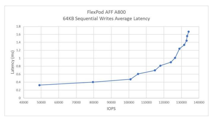
In our testing, we found that the system achieved around 120k IOPS while maintaining under 1ms of serverside latency.
