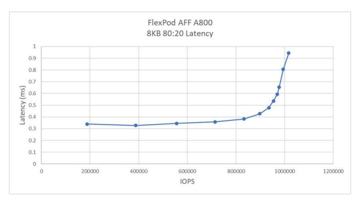
In our testing, we found that the system achieved over 1M IOPS while maintaining just under 1ms of serverside latency.
