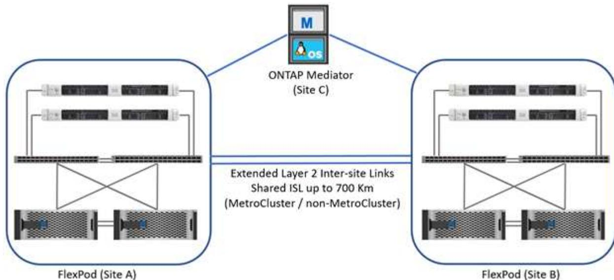
The following two figures depict the VXLAN Multi-Site fabric and the MetroCluster IP storage fabric for a FlexPod MetroCluster IP solution with VXLAN Multi-Site fabric deployment.
