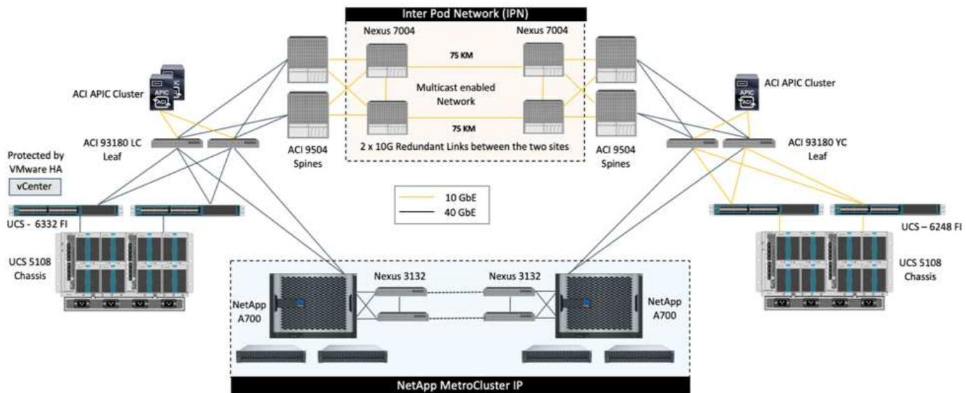
Starting with ONTAP 9.8, ONTAP Mediator can be deployed at a third site to monitor the MetroCluster IP solution and to facilitate automated unplanned switchover when a site disaster occurs.
