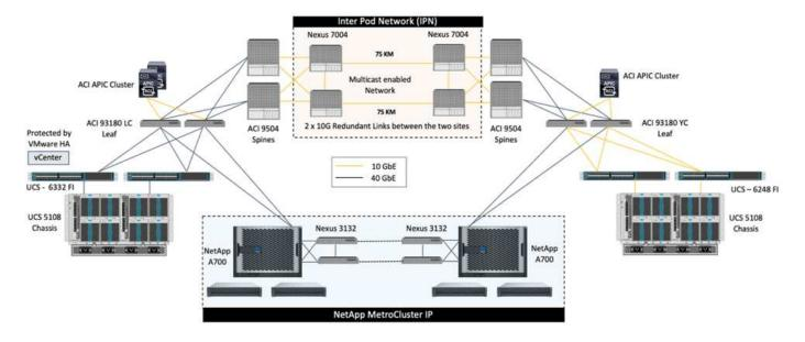
Starting with ONTAP 9.8, ONTAP Mediator can be deployed at a third site to monitor the MetroCluster IP solution and to facilitate automated unplanned switchover when a site disaster occurs.
