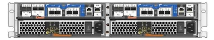
The following figure illustrates 10GBASE-T ports for connection through conventional RJ-45 Ethernet cables.
