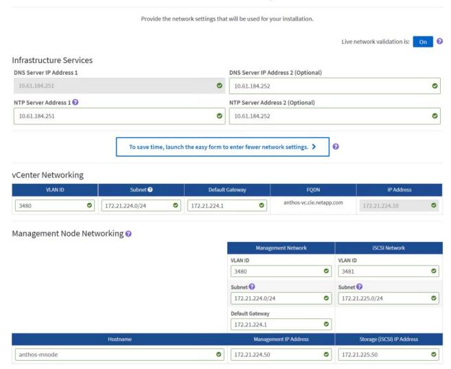
15. The next page allows you to configure each node in the environment. For the compute nodes, it allows you to configure the host name, management network, vMotion network, and storage network. For the storage nodes, name the storage cluster and configure the management and storage networks being used for each node. Click Continue.
