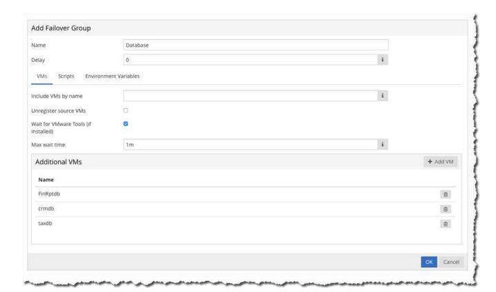
Notice how this example enables Wait for VMware Tools. This setting is important, because it helps make sure that the applications are running. We used the Add VM button to add VMs that are databases. We didn't enable Unregister Source VMs, because it will slow down the failover. We now use the Add Failover button to protect the applications.
