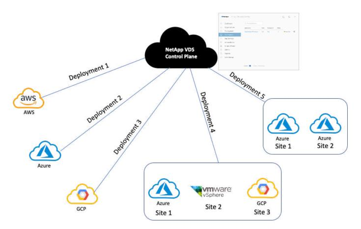
Each deployment is associated with an active directory domain and provides clients with an access entry point for workspaces and applications. A service provider or enterprise that has multiple active directory domains typically has more deployments. A single Active Directory domain that spans multiple regions typically has a single deployment with multiple sites.
