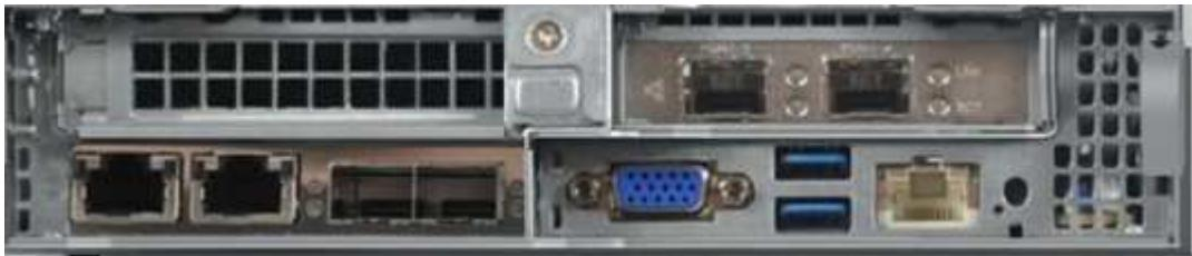
The H610C is 2RU and has a dual-socket first generation Intel Xeon Gold 6130 scalable processor with 16 cores of 2.1GHz, 512GB RAM and two NVIDIA Tesla M10 GPU cards. This server comes with two 10/25GbE SFP28 ports and two 1GbE RJ45 ports, with one 1GbE RJ45 port available for out-of-band management. The following figure depicts a front and back view of an H610C compute node.
