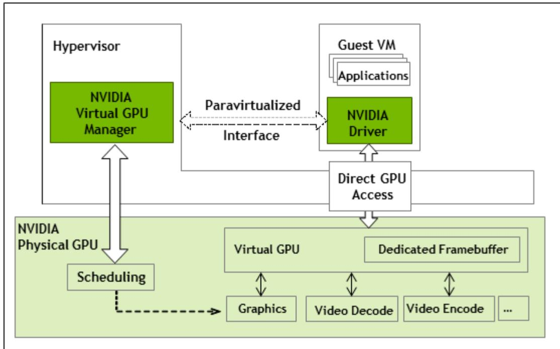
NVIDIA vGPU supports homogenous profiles for each GPU. The placement of virtual machines on a GPU is controlled by a policy that sets either maximum density or maximum performance in response to demand.
