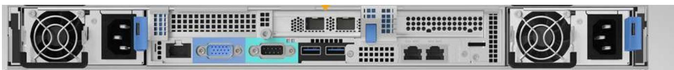
In a single cluster, there can be a mix of storage node models. The capacity of a single node can't exceed 1/3 of the total cluster size. The storage nodes come with two network ports for iSCSI (10/25GbE – SFP28) and two ports for management (1/10GbE – RJ45). A single out-of-band 1GbE RJ45 management port is also available.
