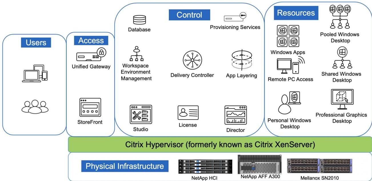
A Mellanox SN2010 switch is used for 10/25/100Gb Ethernet connectivity. Storage nodes use SFP28 transceivers for 25Gb connection, compute nodes use SFP/SFP+ transceivers for 10Gb connection, and interswitch links are QSFP28 transceivers for a 100Gb connection.
