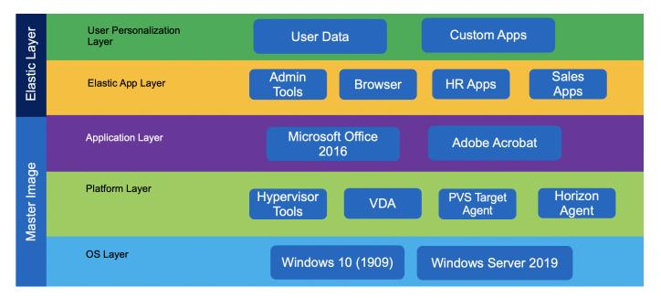
Citrix App Layering uses a single virtual appliance to manage the layers and hands off using the image and application delivery to another platform. The Citrix Enterprise Layer Manager (ELM) portal must be accessed from web browsers that supports Microsoft Silverlight 4.0. A cloud- based management portal is also available if local management interface requirements cannot be met.
