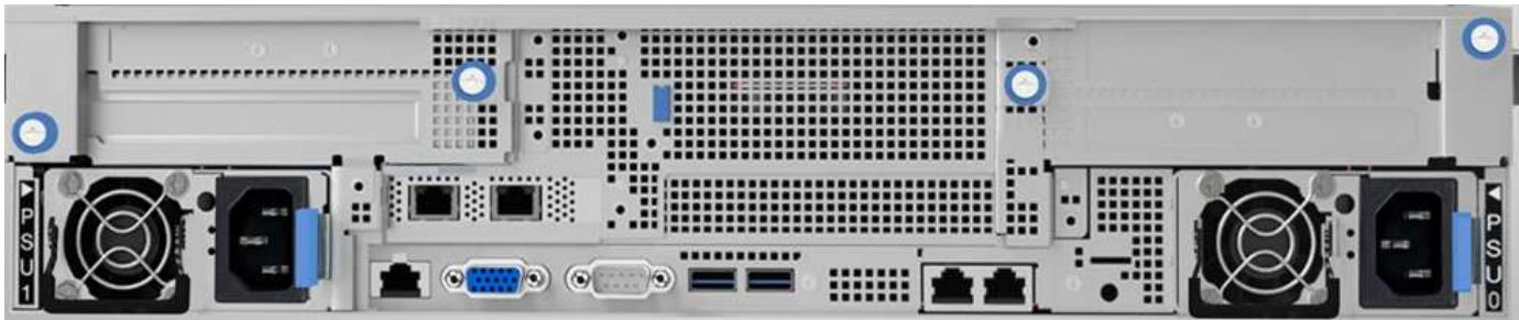
The H610C has two Tesla M10 cards providing a total of 64GB frame buffer memory with a total of 8 GPUs. It can support up to 64 personal virtual desktops with GPU enabled. To host more sessions per server, a shared desktop delivery model is available.
