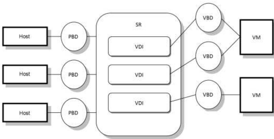
The relationship between the SR and host is handled by a physical block device (PBD), which stores the configuration information required to connect and interact with the given storage target. Similarly, a virtual block device (VBD) maintains the mapping between VDIs and a VM. Apart from that, a VBD is also used for fine tuning the quality of service (QoS) and statistics for a given VDI. The following screenshot presents Citrix Hypervisor storage repository types.
