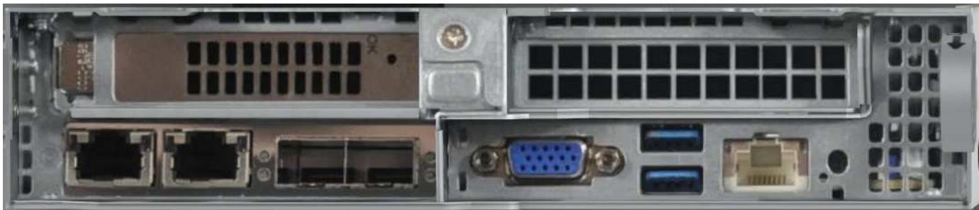
The H610S is a 1U storage node with 12 NVMe drives of sizes 960GB, 1.92TB, or 3.84TB with the option of drive encryption. A minimum of four H610S nodes are required to form a cluster. It delivers around 100,000 IOPS per node with a 4K block size. The following figure depicts a front and back view of an H610S storage node.
