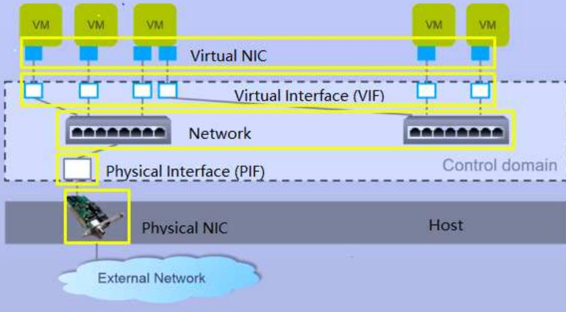
The physical interface (PIF) is associated with a NIC on the server. With Network HCI, up to six NICs are available for use. With the model, which only has two NICs, SR-IOV can be used to add more PIFs. The PIF acts as an uplink port to the virtual switch network. The virtual interface (VIF) connects to a NIC on virtual machines.
