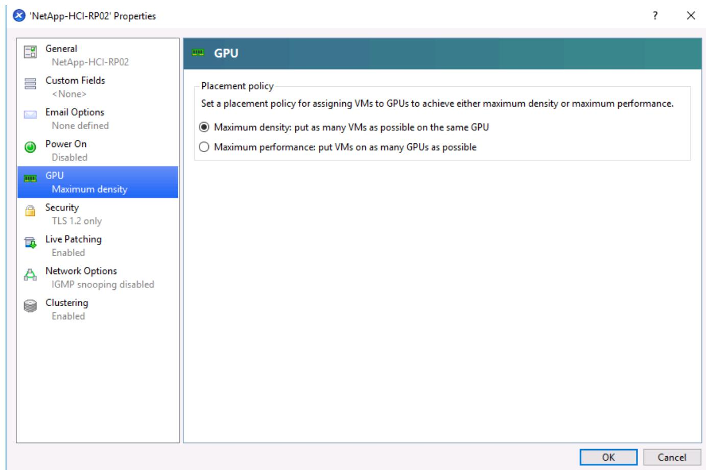
When creating a VM, you can set a virtual GPU profile. The vGPU profile you chose is based on the frame buffer memory level needed, the number of displays, and the resolution requirement. You can also set the
