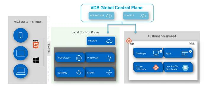
For RDS implementations, NetApp VDS can be readily accessed from Windows and browsers using client software that can be customized to include customer logo and images. Based on user credentials, it provides user access to approved workspaces and applications. There is no need to configure the gateway details.
