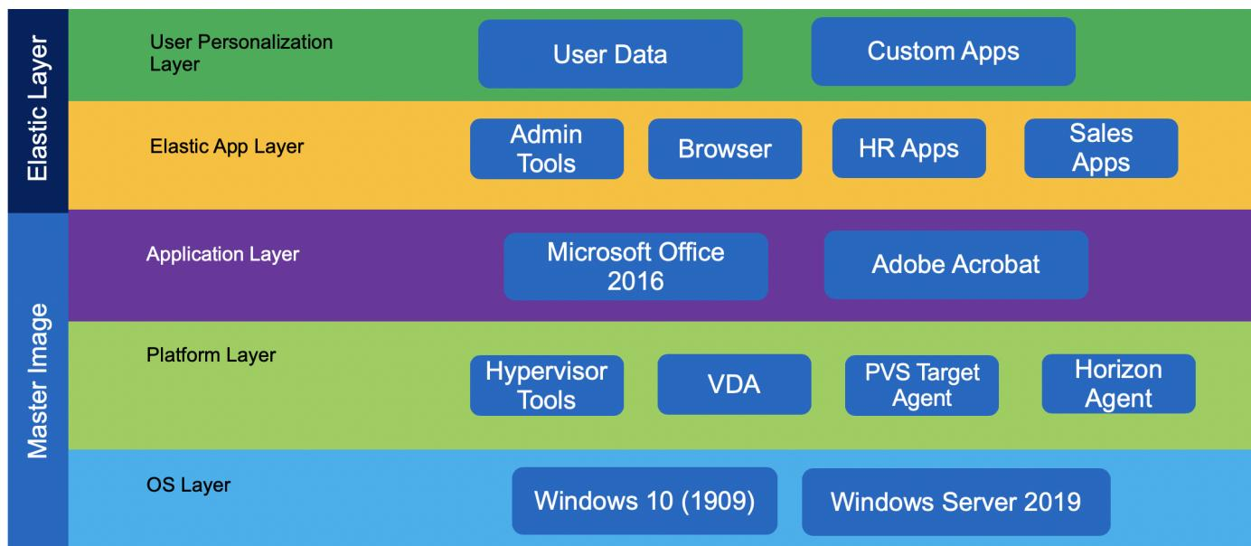
Citrix App Layering uses a single virtual appliance to manage the layers and hands off using the image and application delivery to another platform. The Citrix Enterprise Layer Manager (ELM) portal must be accessed from web browsers that supports Microsoft Silverlight 4.0. A cloud- based management portal is also available if local management interface requirements cannot be met.
