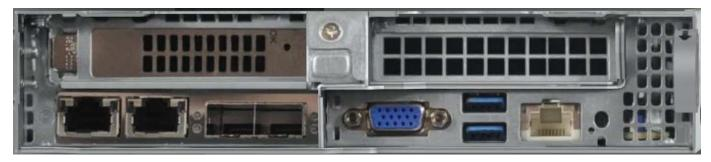
The H610S is a 1U storage node with 12 NVMe drives of sizes 960GB, 1.92TB, or 3.84TB with the option of drive encryption. A minimum of four H610S nodes are required to form a cluster. It delivers around 100,000 IOPS per node with a 4K block size. The following figure depicts a front and back view of an H610S storage node.
