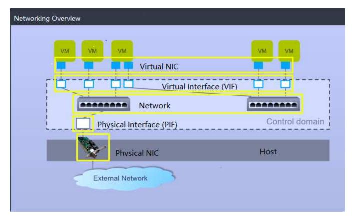
The physical interface (PIF) is associated with a NIC on the server. With Network HCI, up to six NICs are available for use. With the model, which only has two NICs, SR-IOV can be used to add more PIFs. The PIF acts as an uplink port to the virtual switch network. The virtual interface (VIF) connects to a NIC on virtual machines.
