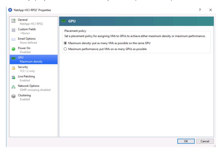
When creating a VM, you can set a virtual GPU profile. The vGPU profile you chose is based on the frame buffer memory level needed, the number of displays, and the resolution requirement. You can also set the
