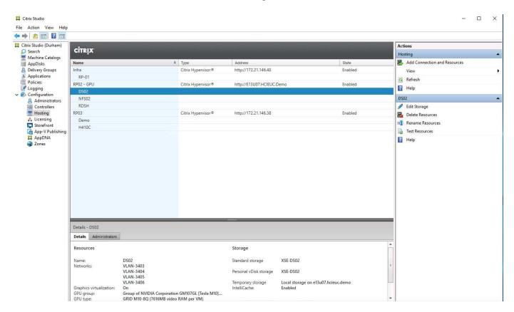
When additional compute capacity is required, a hypervisor server can be added to existing resource pool. Whenever you add a new resource pool and you need to make it available for hosting virtual apps and desktops, you must define a new connection.
