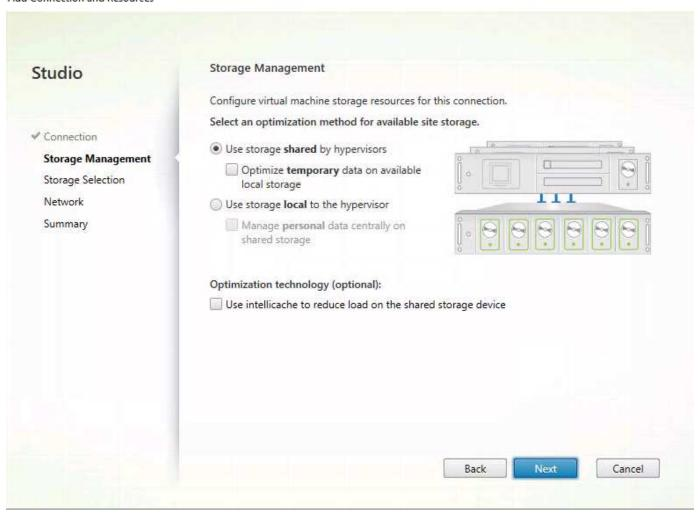
There is also an option to pick resources for the OS, the personal vDisk, and temporary data. When multiple resources are selected, Cltrix Virtual Apps and Desktops automatically spreads the load. In a multitenant environment, a dedicated resource selection can be made for each tenant resource.
