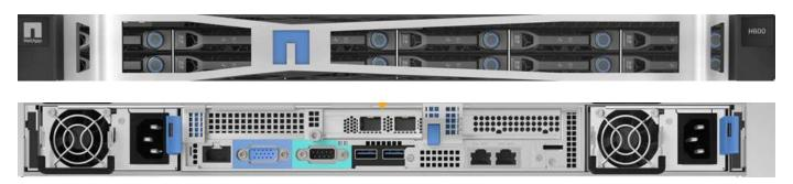
In a single cluster, there can be a mix of storage node models. The capacity of a single node can't exceed 1/3 of the total cluster size. The storage nodes come with two network ports for iSCSI (10/25GbE – SFP28) and two ports for management (1/10/GbE – RJ45). A single out-of-band 1GbE RJ45 management port is also available.
