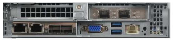
The H610C is 2RU and has a dual- socket first generation Intel Xeon Gold 6130 scalable processor with 16 cores of 2.1GHz, 512GB RAM and two NVIDIA Tesla M10 GPU cards. This server comes with two 10/25GbE SFP28 ports and two 1GbE RJ45 ports, with one 1GbE RJ45 port available for out-of-band management. The following figure depicts a front and back view of an H610C compute node.
