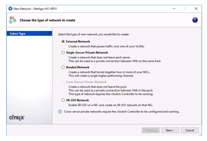
Because the network on Citrix Hypervisor is based on Open vSwitch, you can manage it with ovs-vsctl and ovs-appctl commands. It also supports NVGRE/VXLAN as an overlay solution for large scale- out environments.
