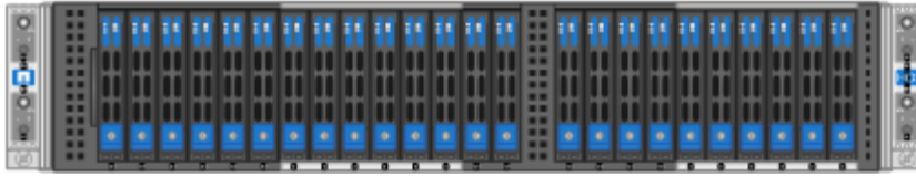
H410S storage nodes in a four-node chassis
