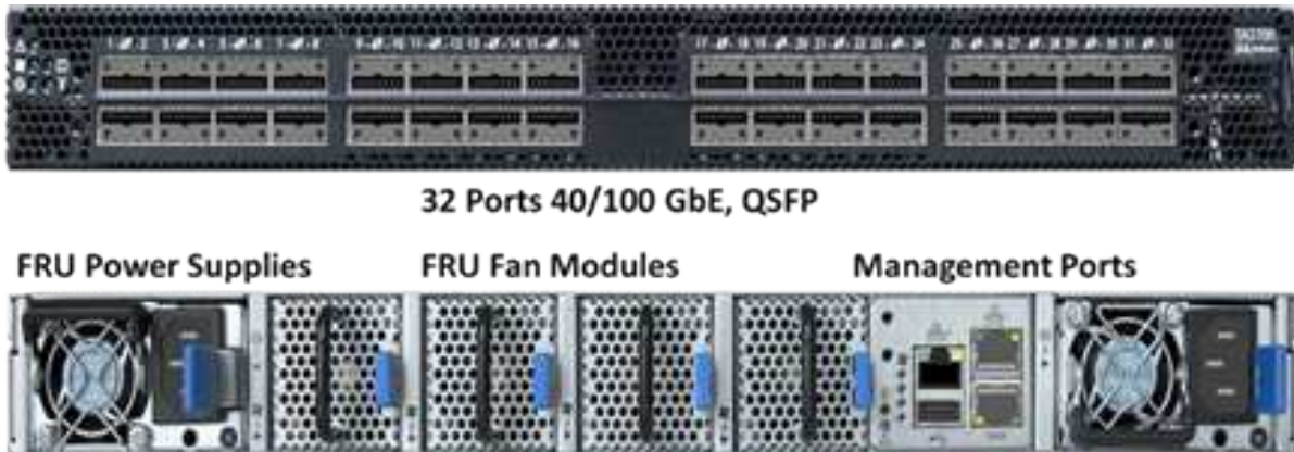
Figure 4: SN2700 switch front and rear
