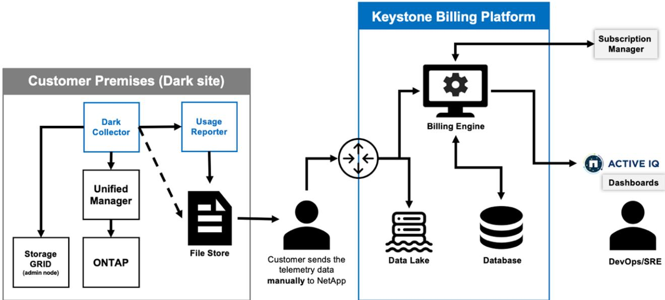
The Keystone Collector service on the server is tasked with periodically gathering usage data, processing this information, and generating a usage file locally on the server. The health service conducts system health checks and is designed to interface with health monitoring systems used by the customer. These reports are available for offline access by users, allowing for validation and aiding in troubleshooting issues.
