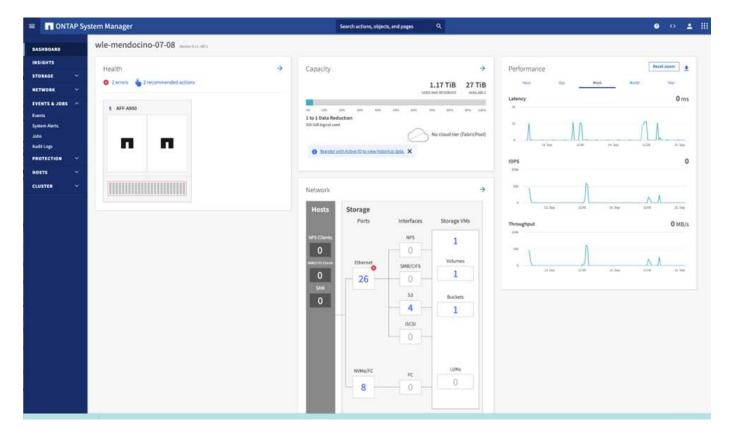
You can configure and manage ONTAP S3 with System Manager and the ONTAP CLI. When you enable S3 and create buckets using System Manager, ONTAP provides best-practice defaults for a simplified configuration. If you configure the S3 server and buckets from the CLI, you can still manage them with System Manager if desired or vice-versa.
