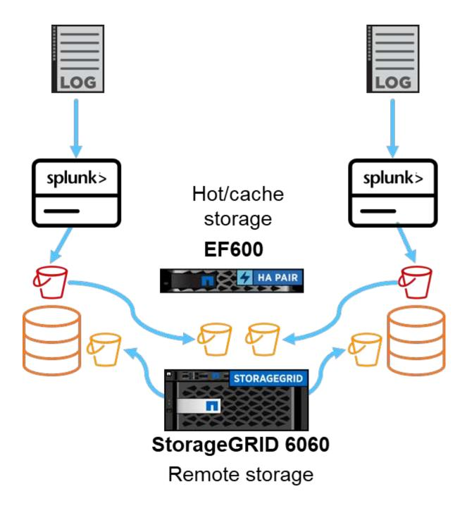
We used EF600 for hot/cache storage and StorageGRID 6060 for remote storage. We used the following architecture for the performance validation. We used two search heads, four heavy forwarders to forward the data to indexers, seven Splunk Event Generators (Eventgens) to generate the real-time data, and 18 indexers to store the data.
