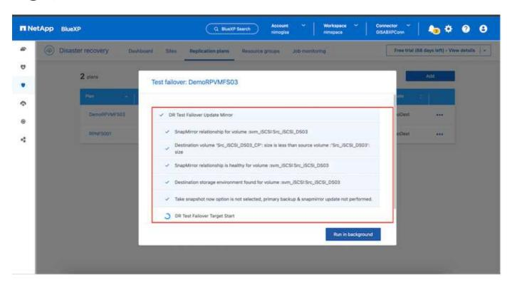
During the process, BlueXP disaster recovery does not map the original target volume. Instead, it makes a new FlexClone volume from the selected Snapshot and a temporary datastore backing the FlexClone volume is mapped to the ESXi hosts.
