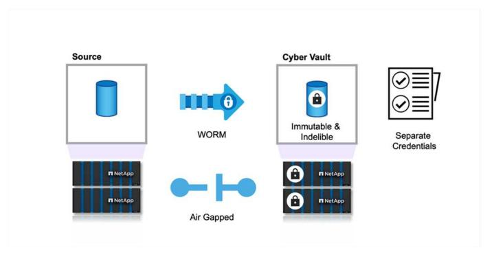
This document describes the automated configuration of NetApp's cyber vault for on-premises ONTAP storage to another designated ONTAP storage with immutable snapshots adding an extra layer of protection from increasing cyber-attacks for rapid recovery. As part of this architecture, the entire configuration is applied as per ONTAP best practices. The last section has instructions for performing a recovery in case of an attack.
