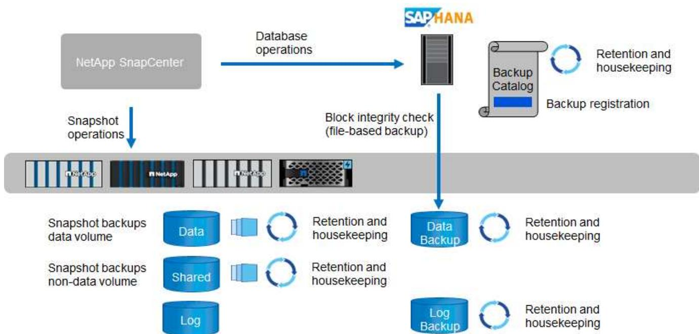
Storage-based Snapshot backups provide significant advantages when compared to conventional file-based backups. These advantages include, but are not limited to, the following:
