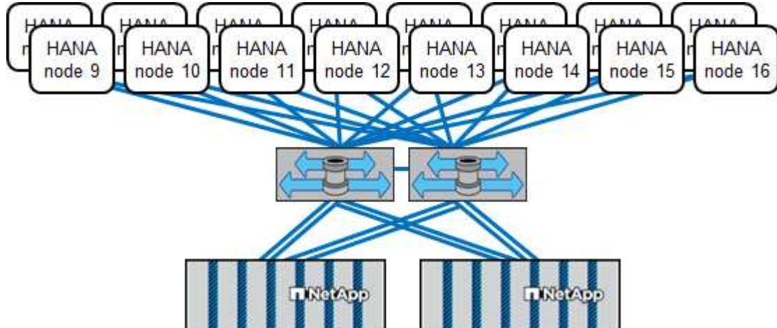
Independent of the deployed AFF system, the SAP HANA landscape can also be scaled by adding any certified storage controllers to meet the desired node density, as shown in the following figure.
