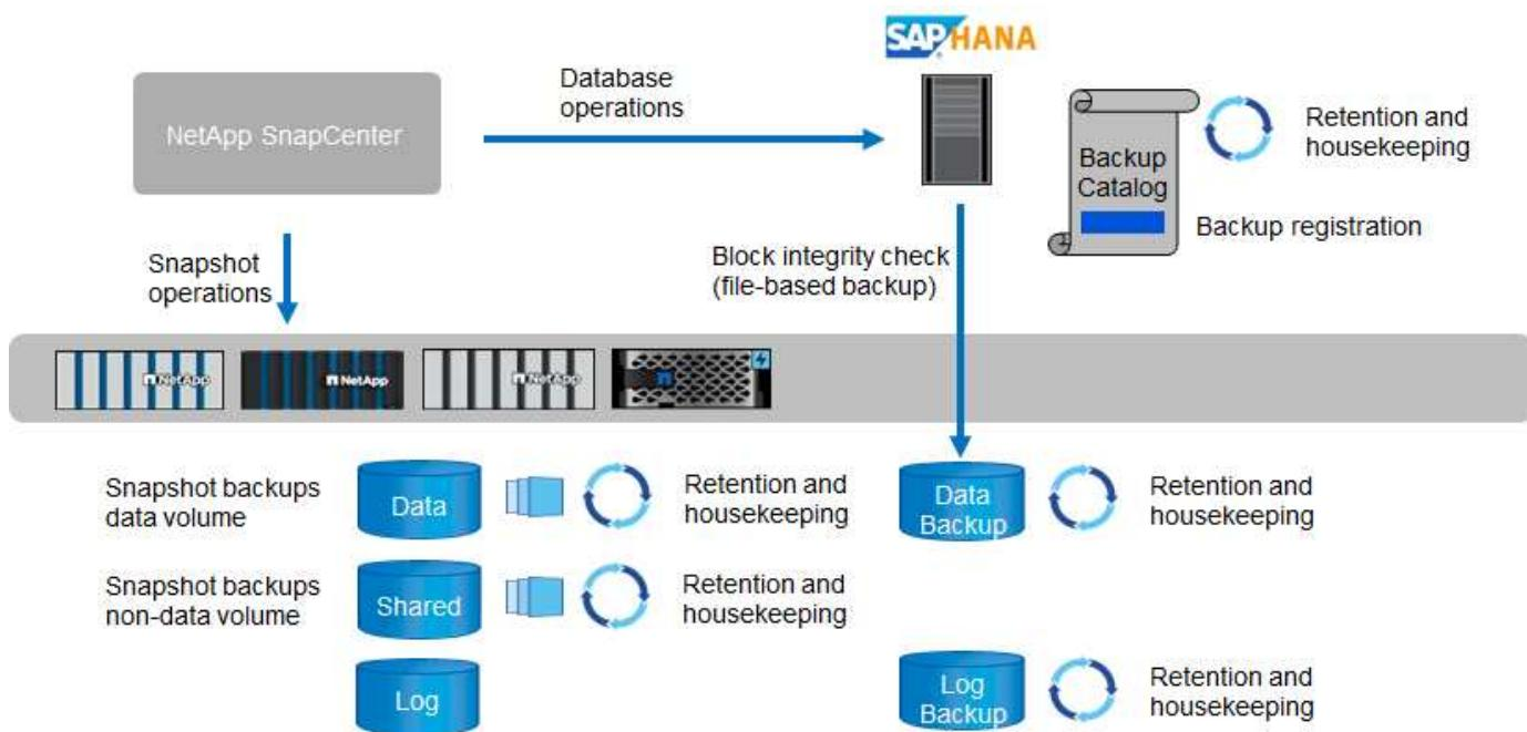
Storage-based Snapshot backups provide significant advantages compared to file-based backups. Those advantages include the following:
