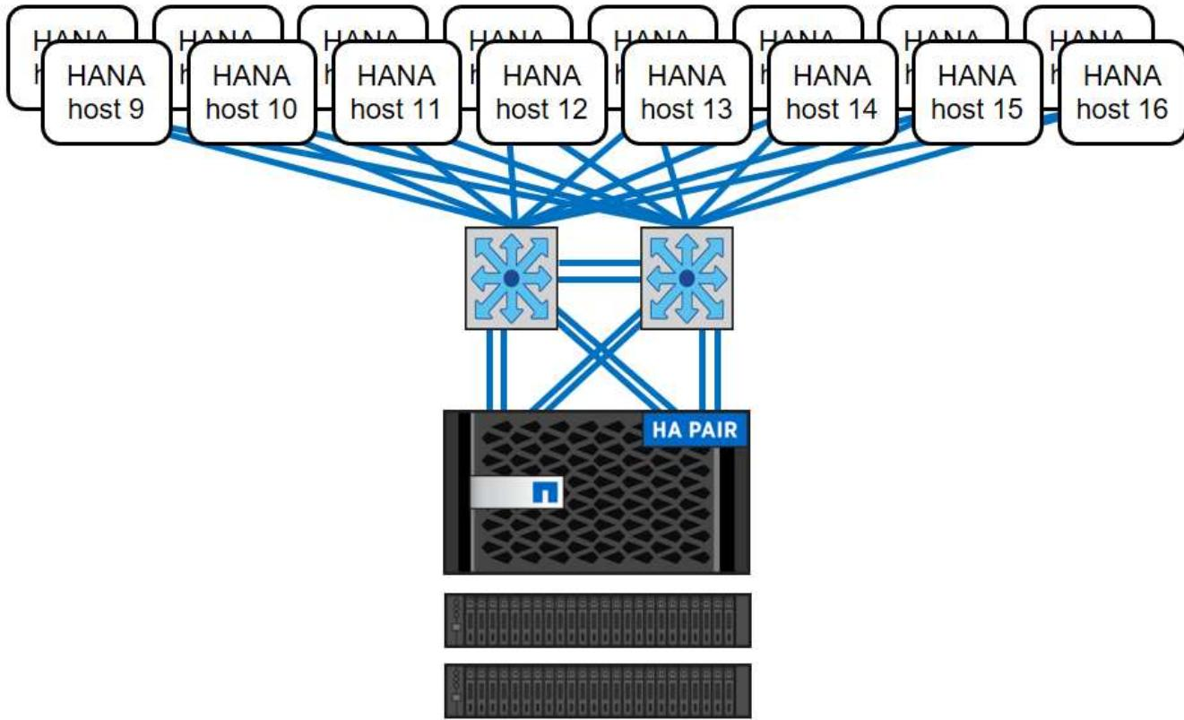
Independent of the deployed FAS system, the SAP HANA landscape can also be scaled by adding any of the certified storage controllers to meet the desired node density (the following figure).
