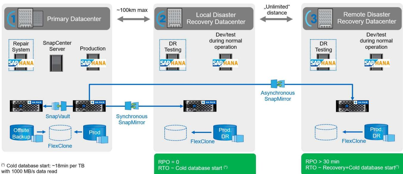
Synchronous replication offers StrictSync mode. If the write to secondary storage is not completed for any reason, the application I/O fails, thereby ensuring that the primary and secondary storage systems are identical. Application I/O to the primary resumes only after the SnapMirror relationship returns to InSync status. If the primary storage fails, application I/O can be resumed on the secondary storage after failover, with no loss of data. In StrictSync mode, the RPO is always zero.
