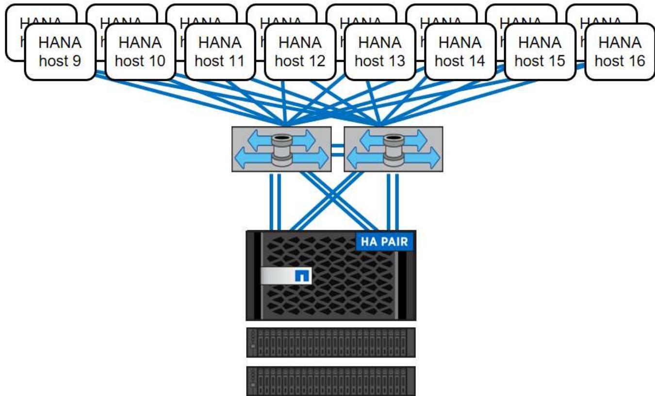
Independent of the deployed FAS system storage model, the SAP HANA landscape can also be scaled by adding more storage controllers, as shown in the following figure.
