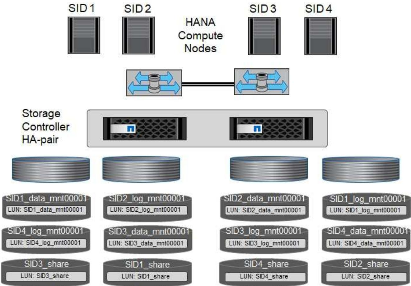
For each SAP HANA host, a data volume, a log volume, and a volume for /hana/shared are configured. The following table shows an example configuration with four SAP HANA single-host systems.
