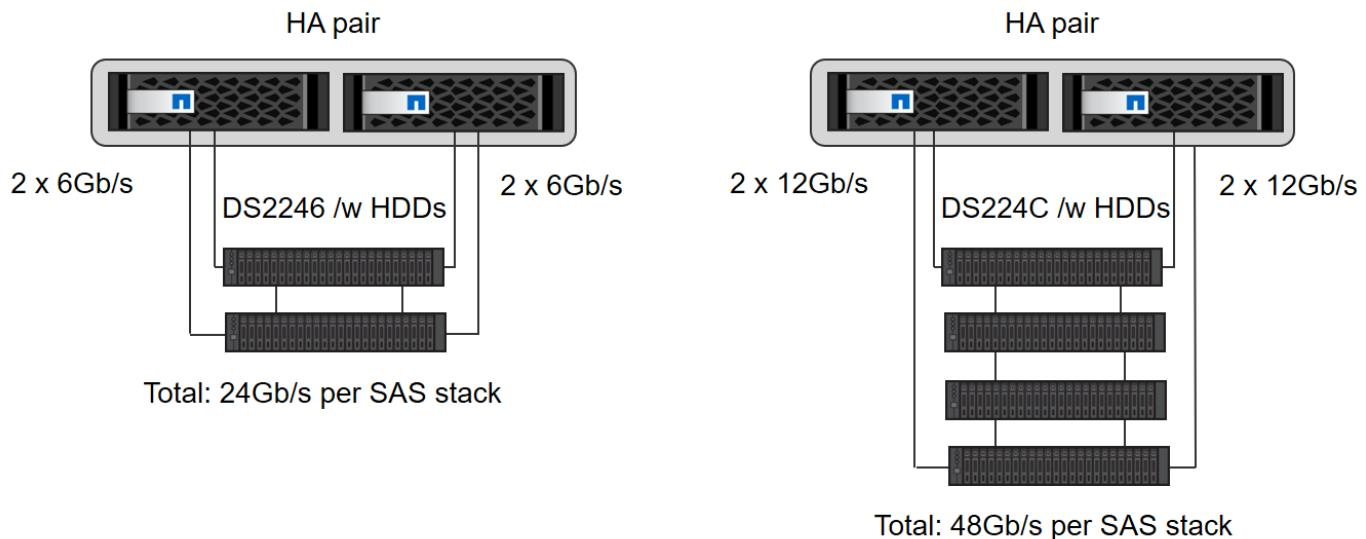
With SSDs, a maximum of one disk shelf can be connected to one SAS stack to provide the required performance for the SAP HANA hosts, as shown in the following figure. The disks within each shelf must be distributed equally to both controllers of the HA pair. With the DS224C disk shelf, quad-path SAS cabling can also be used but is not required.
