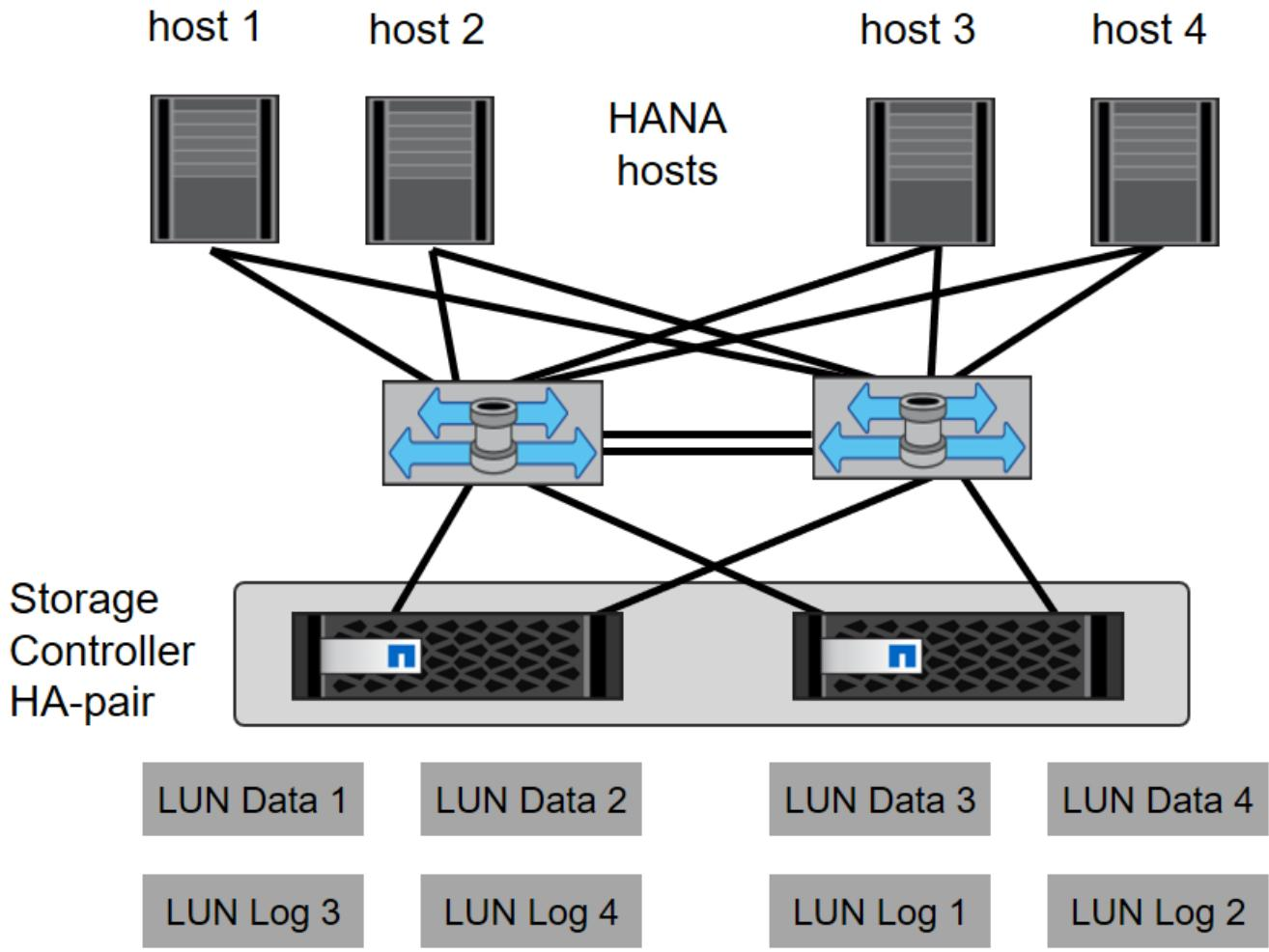
In addition to the zoning on the switch layer, you must map each LUN on the storage system to the hosts that connect to this LUN. Keep the zoning on the switch simple; that is, define one zone set in which all host HBAs can see all controller HBAs.
