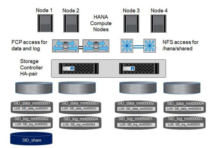
For each SAP HANA host, a data volume and a log volume are created. The /hana/shared volume is used by all hosts of the SAP HANA system. The following figure shows an example configuration for a 4+1 multiple-host SAP HANA system.
