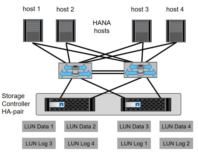
In addition to the zoning on the switch layer, you must map each LUN on the storage system to the hosts that connect to this LUN. Keep the zoning on the switch simple; that is, define one zone set in which all host HBAs can see all controller HBAs.
