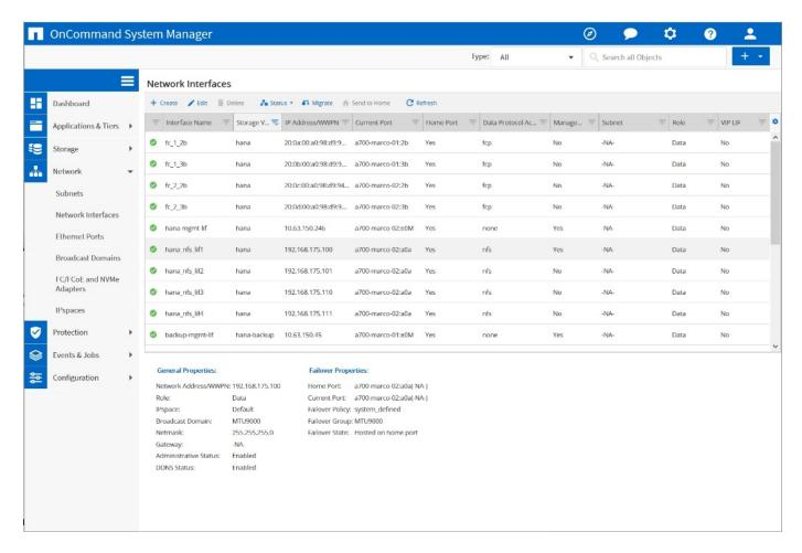
During SVM creation with ONTAP 9.8 System Manager, all the required physical FCP ports can be selected, and one LIF per physical port is created automatically.
