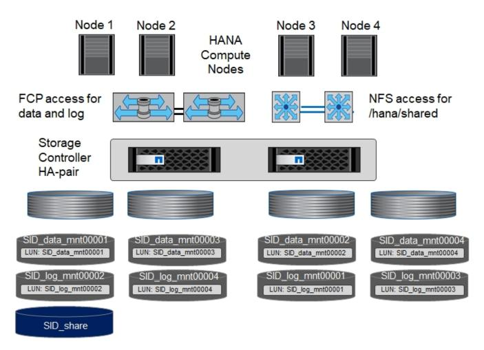
For each SAP HANA host, a data volume and a log volume are created. The <code>/hana/shared</code> volume is used by all hosts of the SAP HANA system. The following figure shows an example configuration for a 4+1 multiple-host SAP HANA system.
