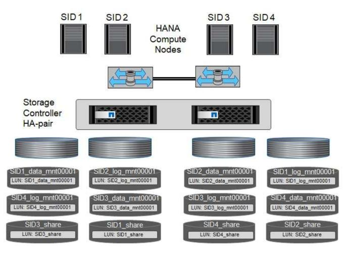
For each SAP HANA host, a data volume, a log volume, and a volume for /hana/shared are configured. The following table shows an example configuration with four SAP HANA single-host systems.
