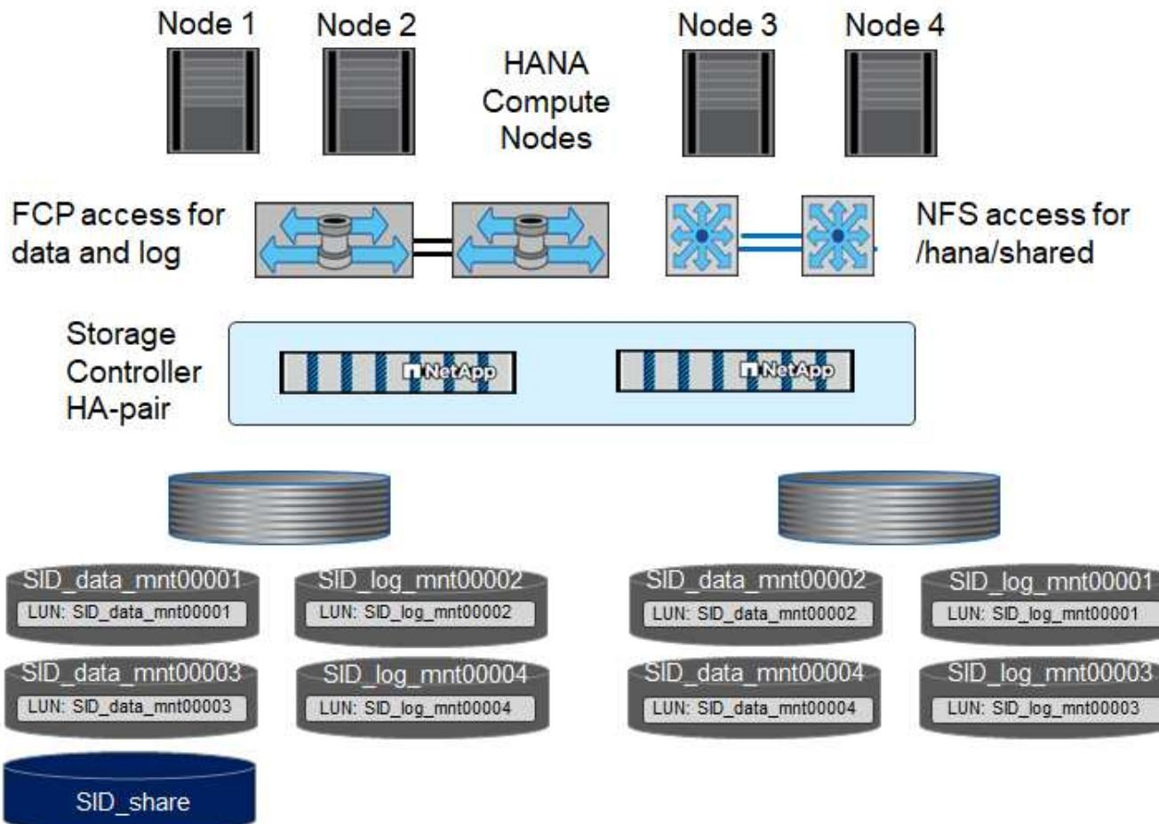
For each SAP HANA host, a data volume and a log volume are created. The /hana/shared volume is used by all hosts of the SAP HANA system. The following table shows an example configuration for a 4+1 multiple-host SAP HANA system.
