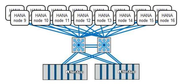
Independent of the deployed AFF system, the SAP HANA landscape can also be scaled by adding any of the certified storage controllers to meet the desired node density, as shown in the following figure.
