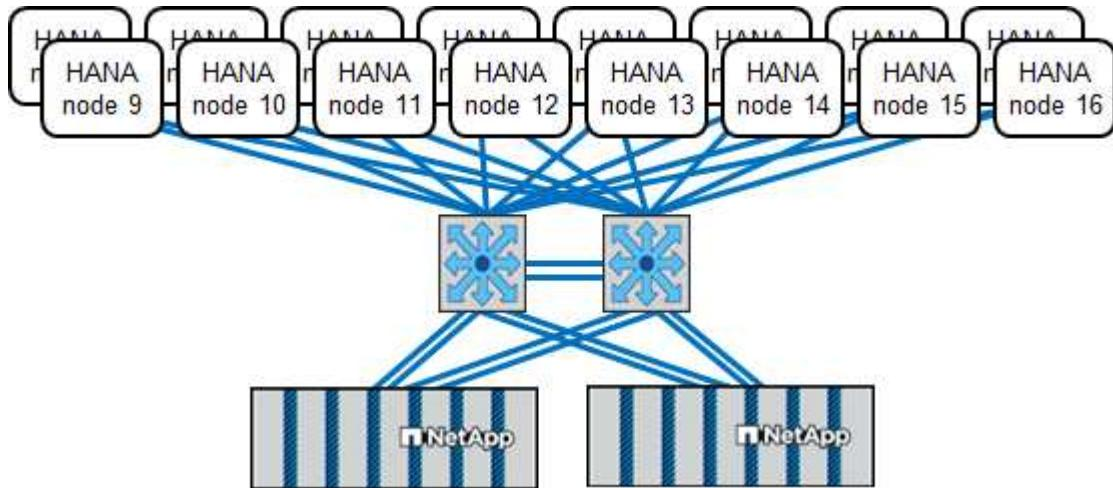
Independent of the deployed AFF system, the SAP HANA landscape can also be scaled by adding any of the certified storage controllers to meet the desired node density, as shown in the following figure.
