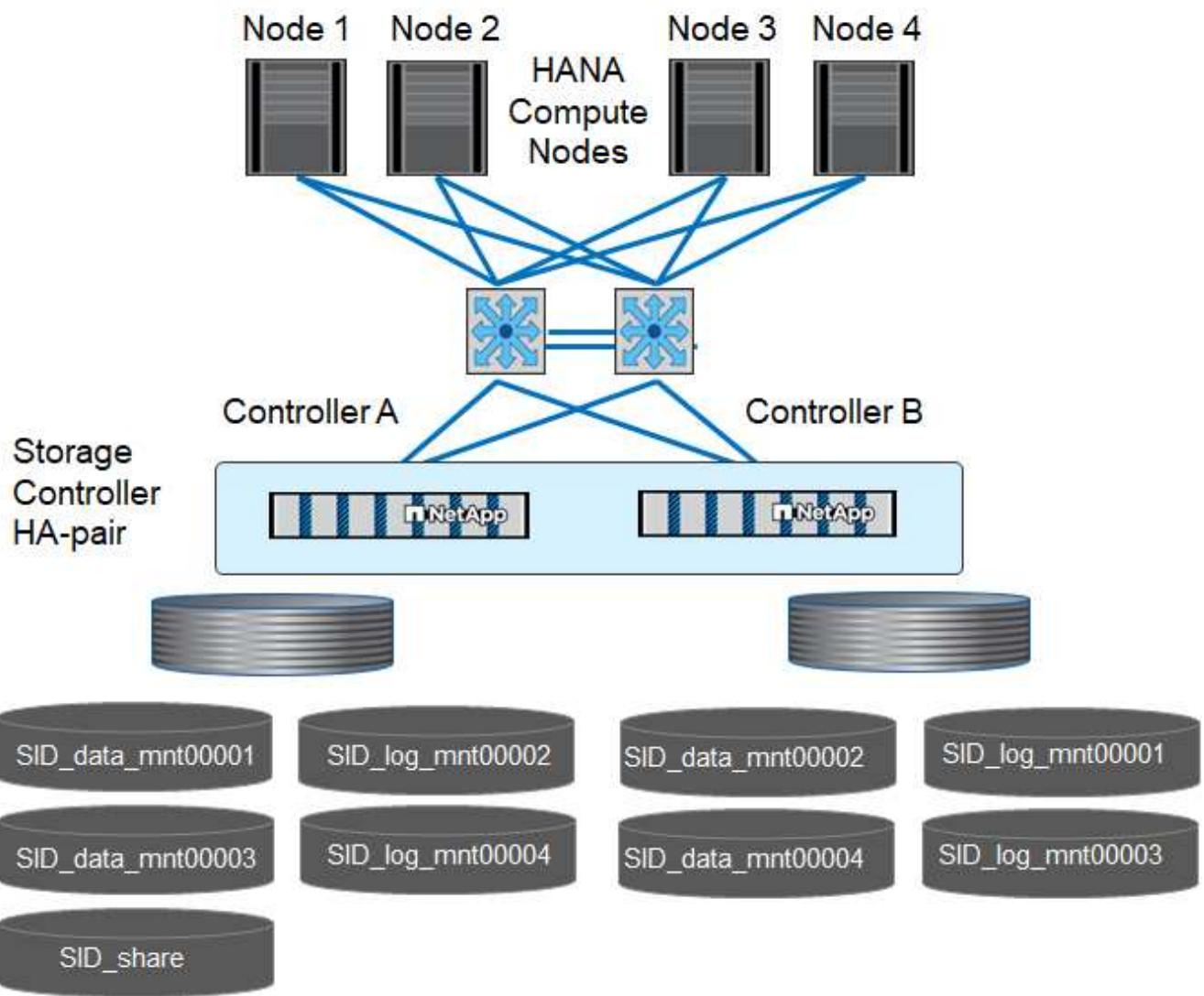
For each SAP HANA host, a data volume and a log volume are created. The /hana/shared volume is used by all hosts of the SAP HANA system. The following table shows an example configuration for a multiple-host SAP HANA system with four active hosts.
