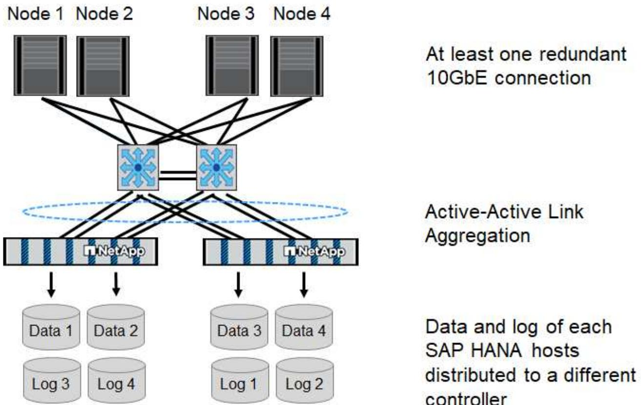
In general, it is recommended to use HA interface groups on the servers (bonds) and the storage systems (for example, Link Aggregation Control Protocol [LACP] and ifgroups). With HA interface groups, verify that the load is equally distributed between all interfaces within the group. The load distribution depends on the functionality of the network switch infrastructure.
