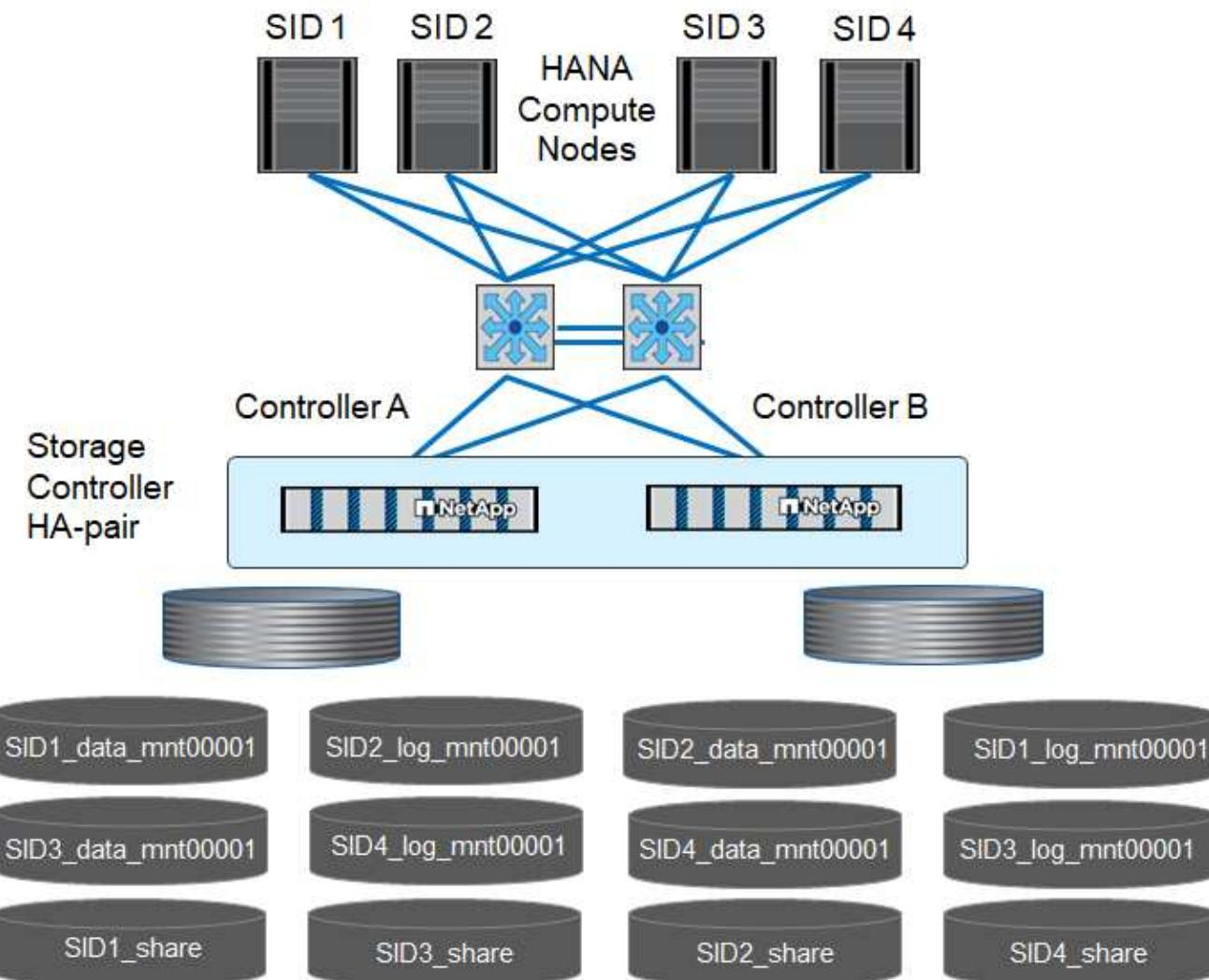
For each SAP HANA host, a data volume, a log volume, and a volume for `/hana/shared` are configured. The following table shows an example configuration for single-host SAP HANA systems.
