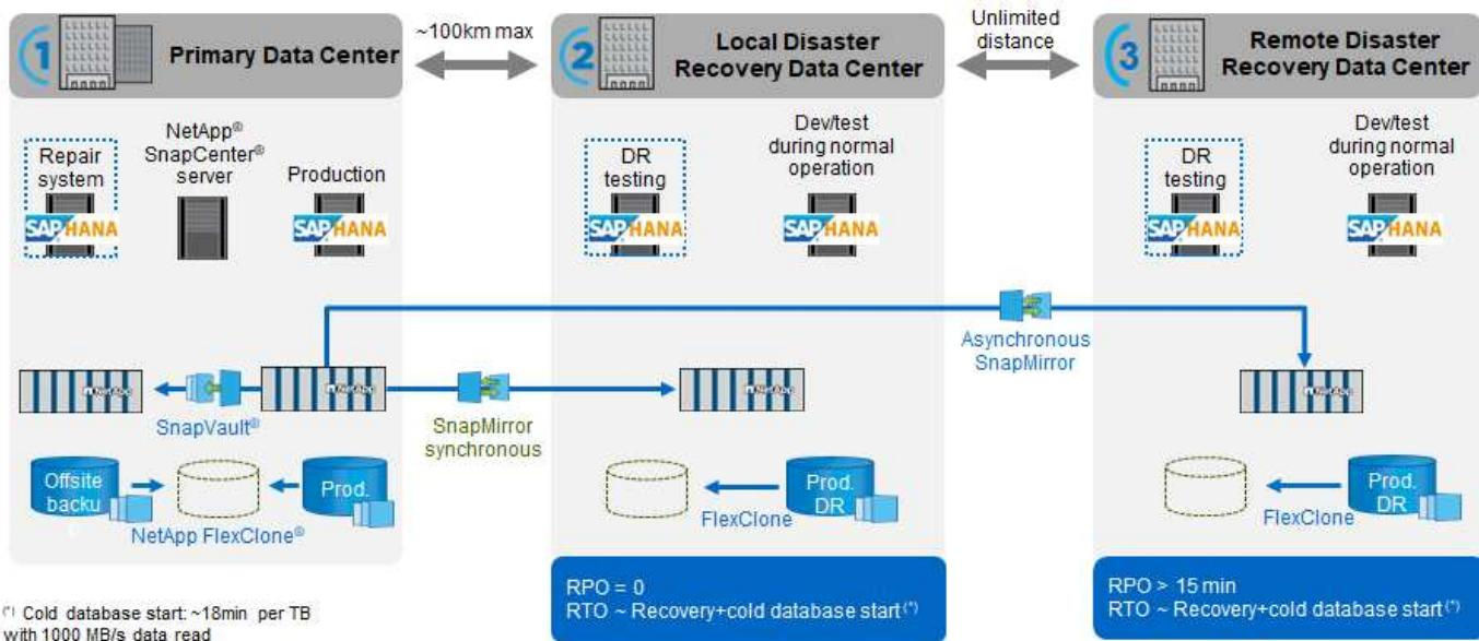
Synchronous replication offers StrictSync mode. If the write to secondary storage is not completed for any reason, the application I/O fails, thereby ensuring that the primary and secondary storage systems are identical. Application I/O to the primary resumes only after the SnapMirror relationship returns to the InSync status. If the primary storage fails, application I/O can be resumed on the secondary storage after failover with no loss of data. In StrictSync mode, the RPO is always zero.
