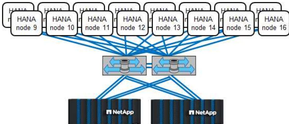
Independent of the deployed ASA system, the SAP HANA landscape can also be scaled by adding any certified storage controllers to meet the desired node density, as shown in the following figure.
