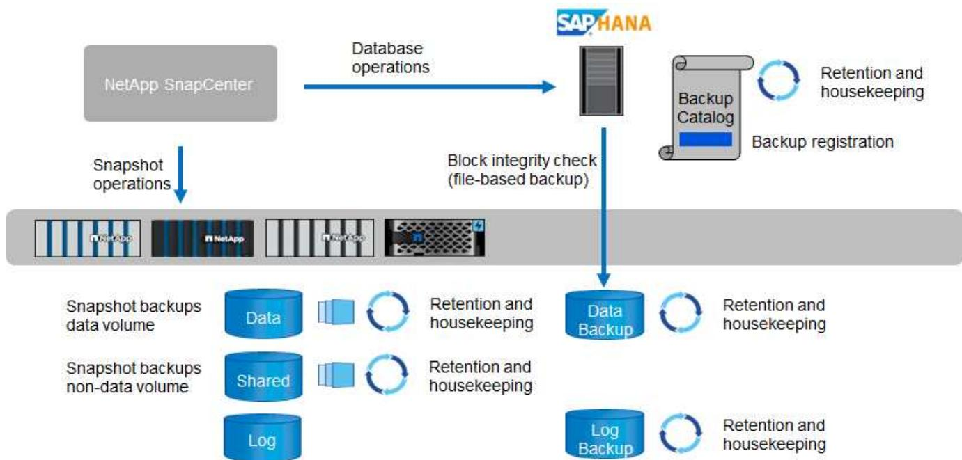
Storage-based Snapshot backups provide significant advantages compared to conventional file-based
