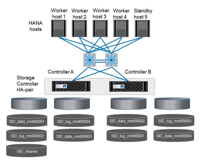
For each SAP HANA host, a data volume and a log volume are created. The <code>/hana/shared</code> volume is used by all hosts of the SAP HANA system. The following table shows an example configuration for a multiple-host SAP HANA system with four active hosts.
