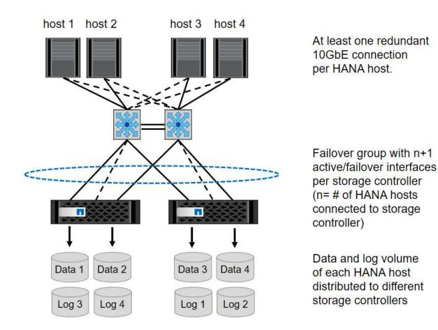
In general, it is also possible to use HA interface groups on the servers (bonds) and the storage systems (for example, Link Aggregation Control Protocol [LACP] and ifgroups). With HA interface groups, verify that the load is equally distributed between all interfaces within the group. The load distribution depends on the functionality of the network switch infrastructure.
