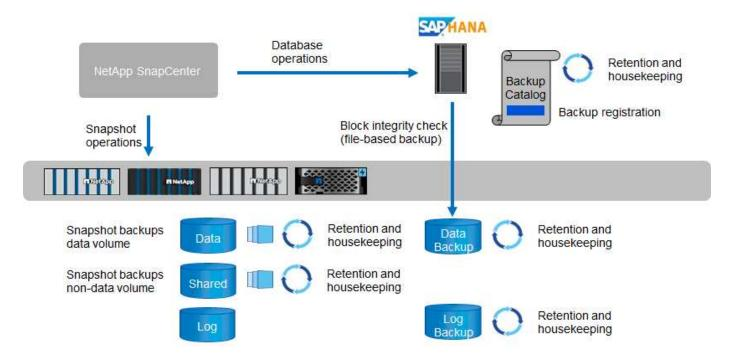
Storage-based Snapshot backups provide significant advantages when compared to conventional file-based backups. These advantages include, but are not limited to, the following:
