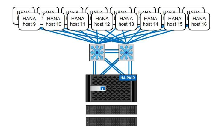
Independent of the deployed FAS system, the SAP HANA landscape can also be scaled by adding any of the certified storage controllers to meet the desired node density (the following figure).
