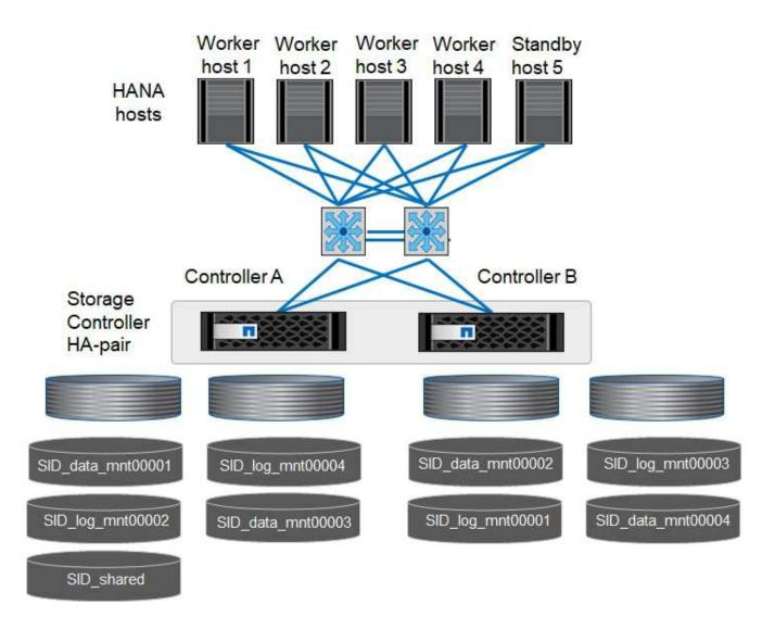
For each SAP HANA host, a data volume and a log volume are created. The /hana/shared volume is used by all hosts of the SAP HANA system. The following table shows an example configuration for a multiple-host SAP HANA system with four active hosts.
