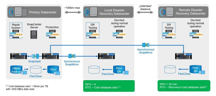
Synchronous replication offers StrictSync mode. If the write to secondary storage is not completed for any reason, the application I/O fails, thereby ensuring that the primary and secondary storage systems are identical. Application I/O to the primary resumes only after the SnapMirror relationship returns to InSync status. If the primary storage fails, application I/O can be resumed on the secondary storage after failover, with no loss of data. In StrictSync mode, the RPO is always zero.
