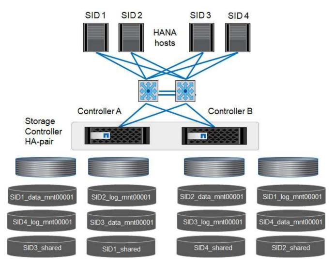
For each SAP HANA DB host, a data volume, a log volume, and a volume for /hana/shared are configured. The following table shows an example configuration for single-host SAP HANA systems.
