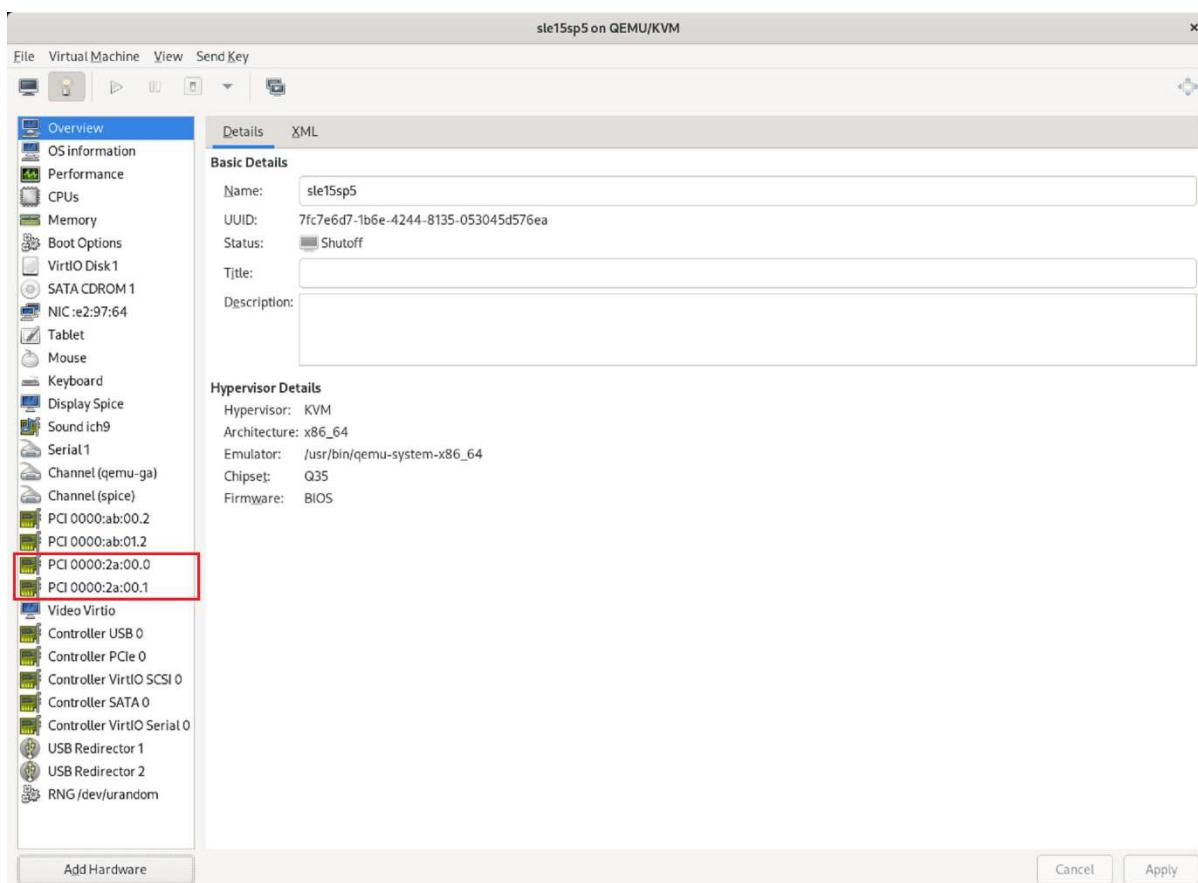
Physical ports are passed through to the VM, so no additional preparation is required within the VM.
