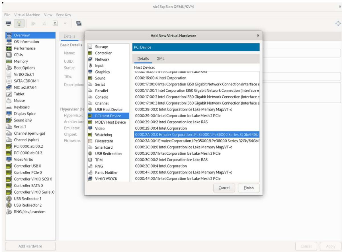
5. Choose the desired HBA port from the list of PCI Host Device belonging to the second fabric and press finish. In this example 0000.A2:00:1.
