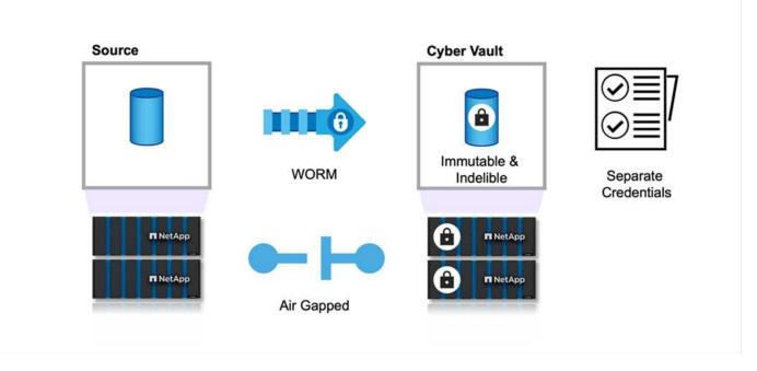
This document describes the automated configuration of NetApp's cyber vault for on-premises ONTAP storage to another designated ONTAP storage with immutable snapshots adding an extra layer of protection from increasing cyber-attacks for rapid recovery. As part of this architecture, the entire configuration is applied as per ONTAP best practices. The last section has instructions for performing a recovery in case of an attack.
