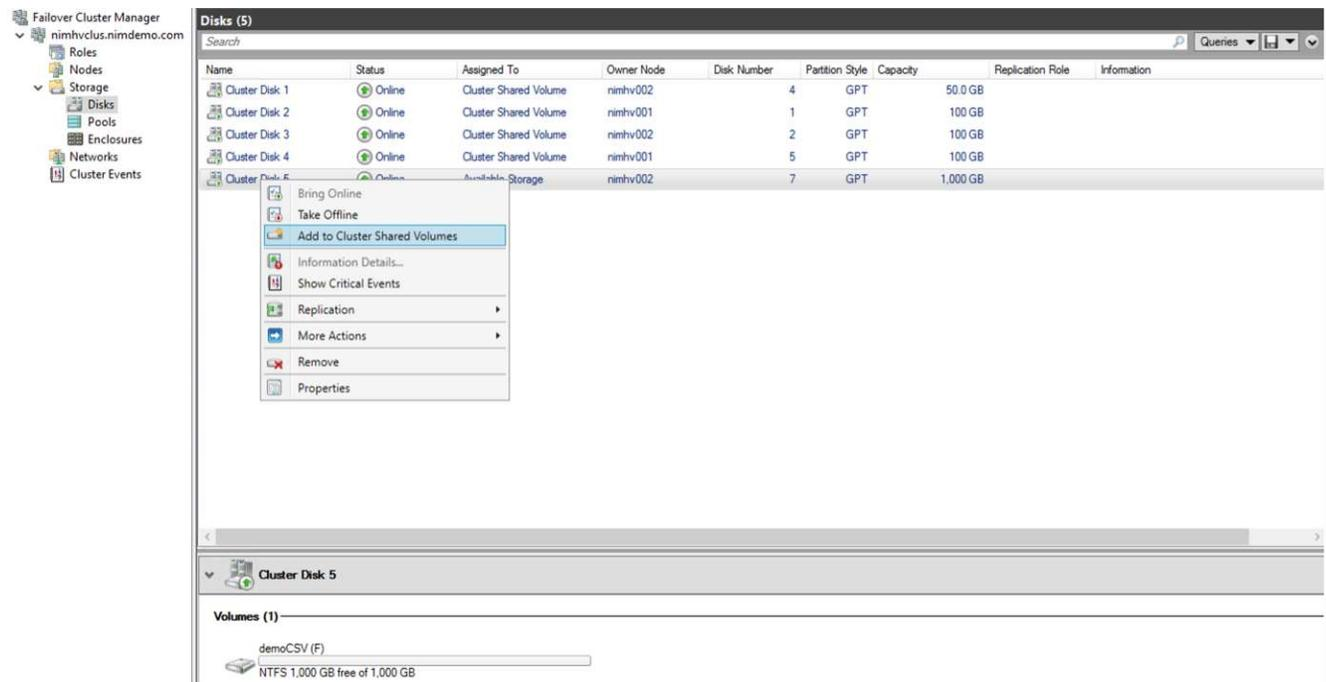
6. The disks are now assigned to the Cluster Shared Volume group in the cluster. The disks are exposed to each cluster node as numbered volumes (mount points) under the %SystemDrive%\ClusterStorage folder. The volumes appear in the CSVFS file system.
