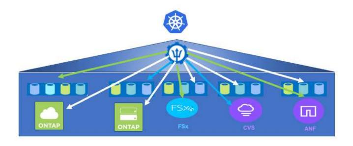
ONTAP Storage Virtual Machine (SVM) provides secure multi-tenancy. A Single OpenShift cluster can connect to single SVM or multiple SVMs or even to multiple ONTAP clusters. Storage class filters the backend storage based on parameters or by labels. Storage administrators define the parameters to connect to storage system using trident backend configuration. On successful connection establishment, it creates the trident backend and populates the information which the storage class can filter.
