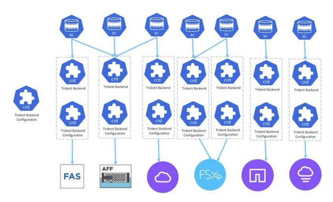
Application owner requests persistent volume using storage class. The storage class filters the backend storage.
