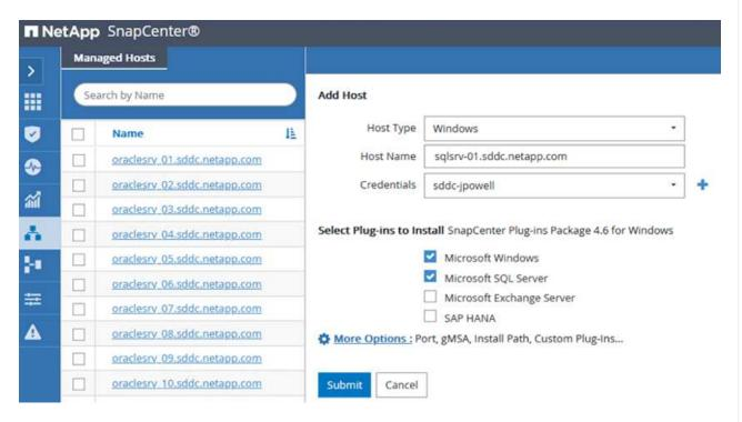
For Oracle, fill out the required fields in the Add Host dialog box and select the check box for the Oracle Database plug-in. Then click Submit to begin the discovery process and to add the host to SnapCenter.
