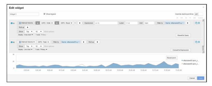
The chart displays the total IOPS as a line, with the chart showing the combination of read and write IOPS in blue. The gap between 9:30 and 9:45 shows non-read and non-write IO (overhead) operations.
