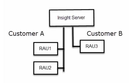
You need to create individual keys for each customer in this configuration. Customer A requires identical keys for both RAUs. Customer B requires a single set of keys.
