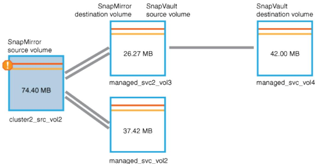
5. You place your cursor over the error icon to see the pop-up dialog box that displays the threshold settings and see that the volume has exceeded the error threshold, indicating a capacity issue.
