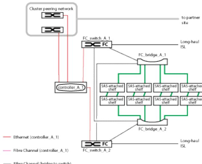
A two-node configuration includes the following connections:
