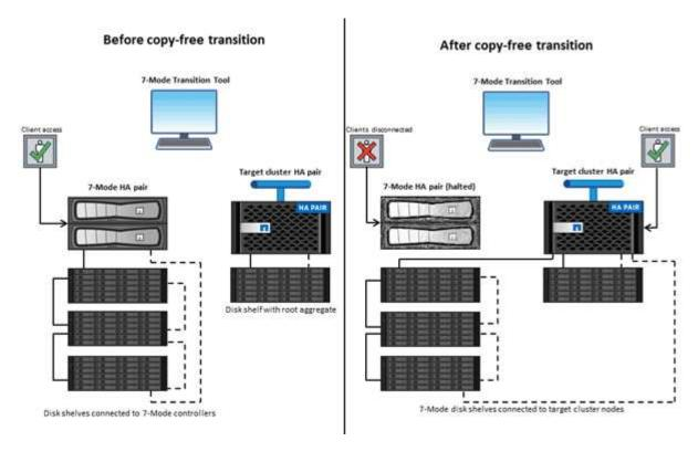
The 7-Mode Transition Tool runs on a Windows system and provides web interface for managing transition operations.
