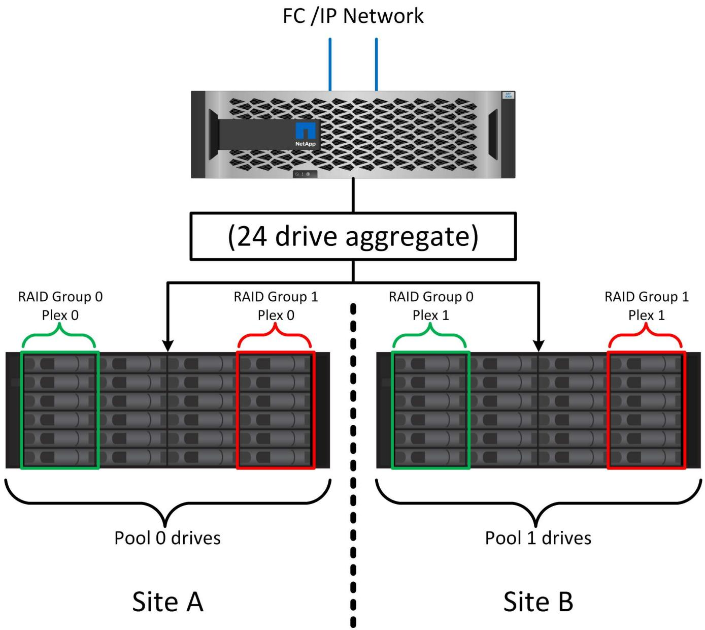
The figure above illustrates a sample SyncMirror configuration. A 24-drive aggregate was created on the controller with 12 drives from a shelf allocated on site A and 12 drives from a shelf allocated on site B. The drives were grouped into two mirrored RAID groups. RAID group 0 includes a 6-drive plex on site A mirrored to a 6-drive plex on site B. Likewise, RAID group 1 includes a 6-drive plex on site A mirrored to a 6-drive plex on site B.
