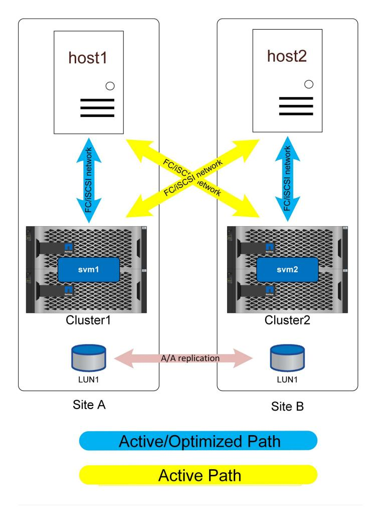
In normal operation, all IO is local IO. Reads and writes are serviced from the local storage array. Write IO will, of course, also need to be replicated by the local controller to the remote system before being acknowledged, but all read IO will be serviced locally and will not incur extra latency by traversing the SAN link between sites.
