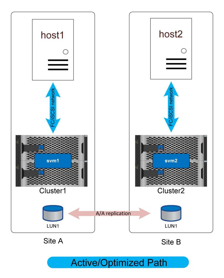
An ASA configuration with non-uniform access would work largely the same as it would with AFF. With uniform access, IO would be crossing the WAN. This may or may not be desirable.
