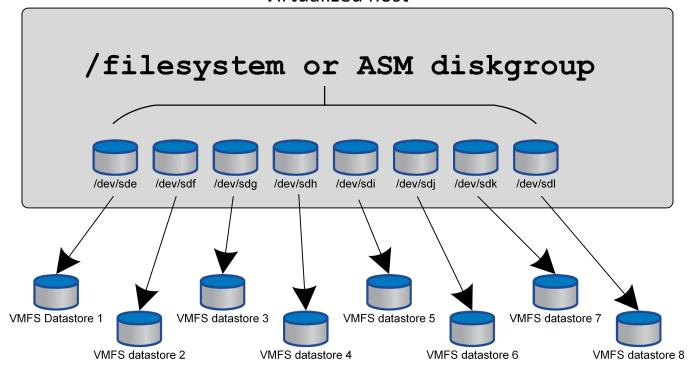
The primary driver for this approach is not ONTAP, it's because of inherent limitation of the number of operations a single VM or hypervisor LUN can service in parallel. A single ONTAP LUN can generally support far more IOPS than a host can request. The single-LUN performance limit is almost universally a result of the host OS. The result is that most databases need between 4 and 8 LUNs to meet their performance needs.
