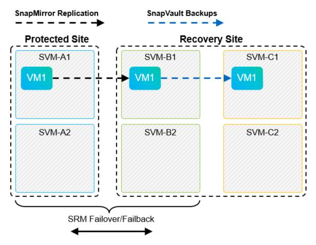
The following figure depicts the configuration after SRM has been used to reverse SnapMirror replication back to the primary site. The environment has also been reconfigured such that SnapVault backups are occurring from what is now the SnapMirror source. This setup is a SnapMirror SnapVault fan-out configuration.
