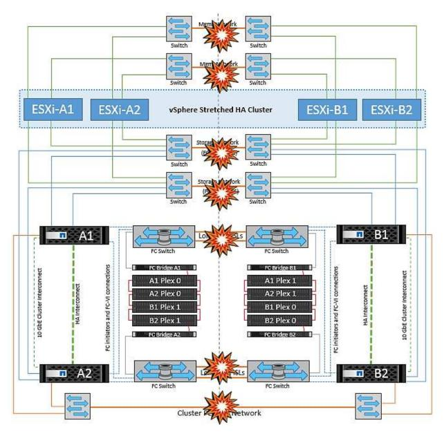
NetApp recommends determining if any virtual machine has violated the DRS rules. Any virtual machines running from a remote site will be down since they will not be able to access the datastore, and vSphere HA will restart that virtual machine on the local site. After the ISL links are back online, the virtual machine that was running in the remote site will be killed, since there cannot be two instances of virtual machines running with the same MAC addresses.
