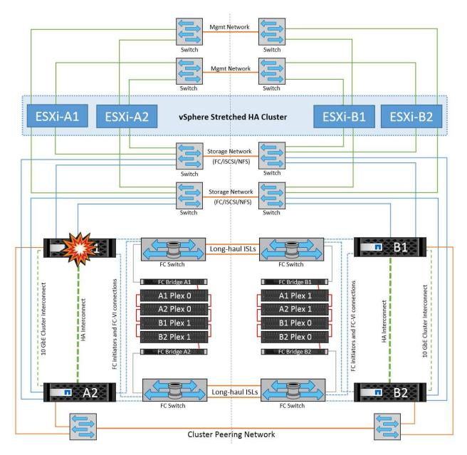
If the failover is part of a rolling disaster (node A1 fails over to A2), and there is a subsequent failure of A2, or the complete failure of site A, switchover following a disaster can occur at site B.
