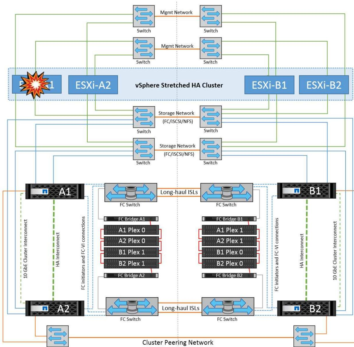
In this scenario, if there is an ESXi host failure, the master node in the VMware HA cluster detects the host failure since it no longer receives network heartbeats. To determine whether the host is really down or only a network partition, the master node monitors the datastore heartbeats and, if they are absent, it performs a final
