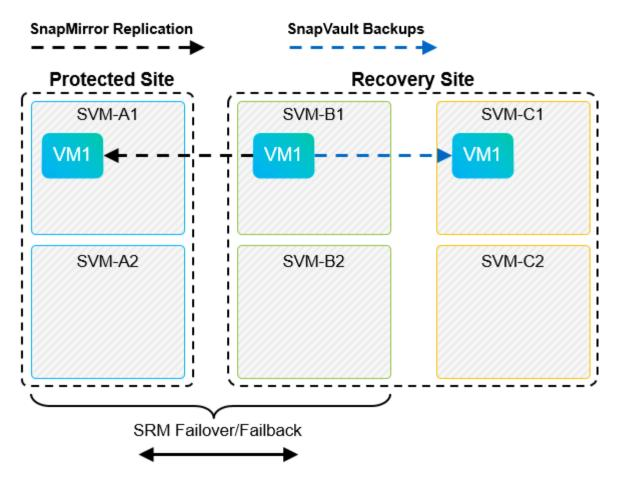
After SRM performs failback and a second reversal of the SnapMirror relationships, the production data is back at the primary site. This data is now protected in the same way that it was before the failover to the DR site—through SnapMirror and SnapVault backups.
