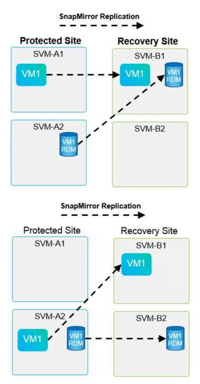
Any replication relationship in which an individual NetApp volume is replicated from one source SVM to multiple destinations in the same SVM or in different SVMs is referred to as SnapMirror fan-out. Fan-out is not supported with SRM. In the example shown in the following figure, VM1 cannot be configured for protection in SRM because it is replicated with SnapMirror to two different locations.
