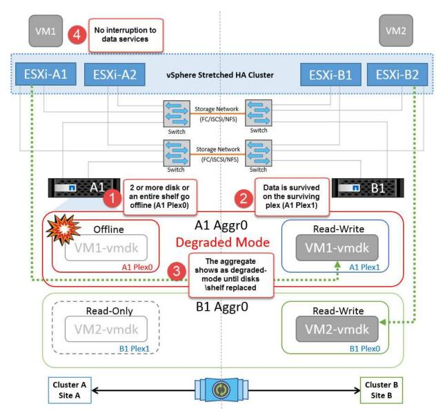
**Note:** During this period, there is no impact on the virtual machine I/O operations, but there is degraded performance because the data is being accessed from the remote disk shelf through ISL links.
