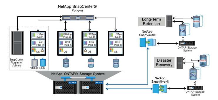
For enhanced disaster recovery capabilities, consider using the NetApp SRA for ONTAP with VMware Site Recovery Manager. In addition to support for the replication of datastores to a DR site, it also enables nondisruptive testing in the DR environment by cloning the replicated datastores. Recovery from a disaster and reprotecting production after the outage has been resolved are also made easy by automation built into SRA.
