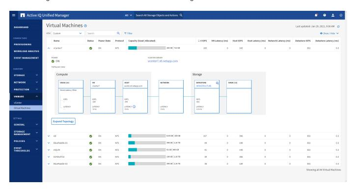
Unified Manager presents the underlying sub-system of a virtual environment in a topological view for determining whether a latency issue has occurred in the compute node, network, or storage. The view also highlights the specific object that causes the performance lag for taking remedial steps and addressing the underlying issue.
