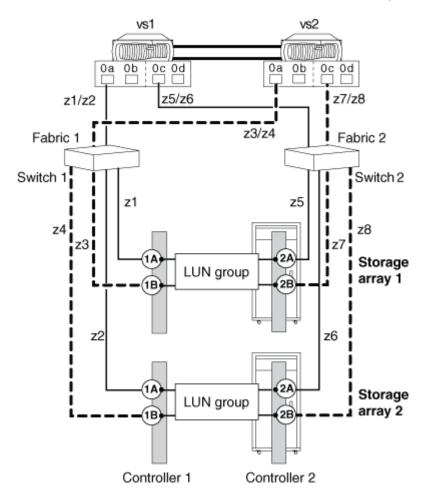
The following table shows the 1:1 zoning definitions for the example of one FC initiator port sharing multiple target ports on different storage arrays.
