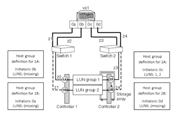
The following example shows the storage array config show output for the illustrated situations where the ONTAP system is zoned to the storage array but there are no LUNs in the host group definitions for the storage controller 1A, resulting in an open target port. The controllers 1B and 2B do not have LUNs in their respective host group definitions, resulting in an empty host group.
