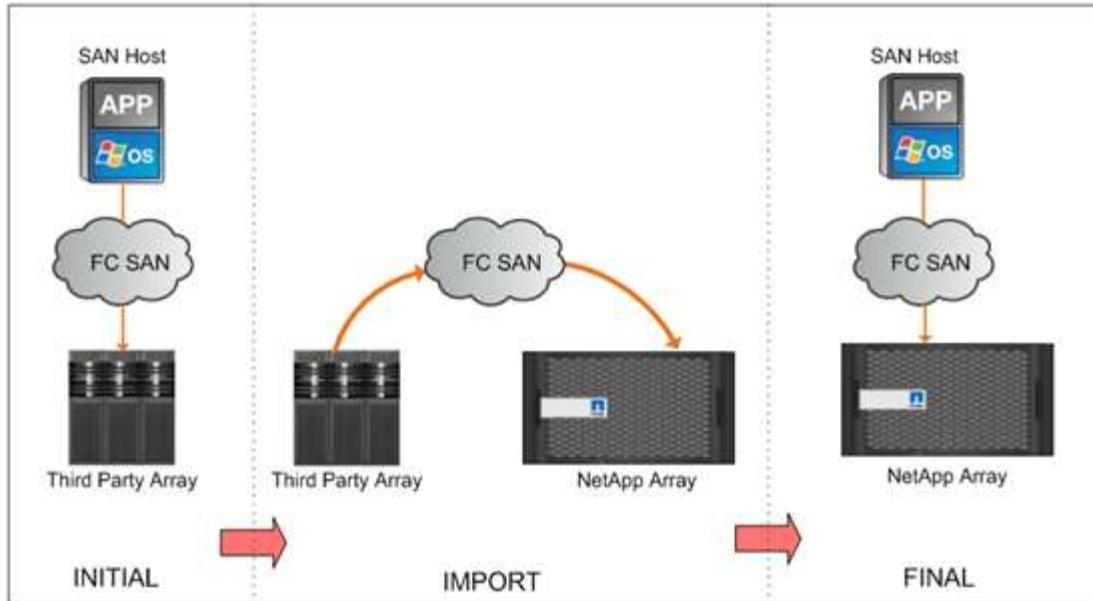
This figure shows an FLI online data migration. The host is connected to the NetApp controller where the new LUN is now hosted. Host operation can then resume and continue during the import.
