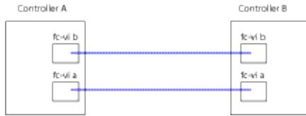
The above illustration is a typical representation of the required cabling. The specific FC-VI ports vary by controller module.
