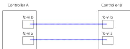
The above illustration is a typical representative cable connection. The specific FC-VI ports will vary by controller module.
