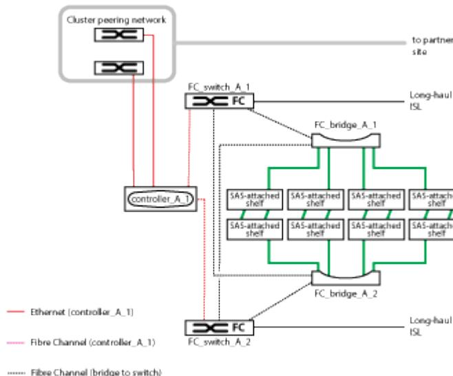
A two-node configuration includes the following connections:
