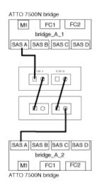
2. For additional shelf stacks, repeat the previous steps using the next available SAS port on the FibreBridge bridges, using port B for a second stack, port C for a third stack, and port D for a fourth stack.
