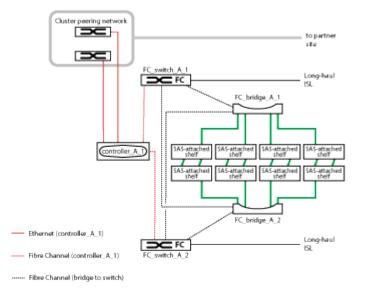
A two-node configuration includes the following connections:
