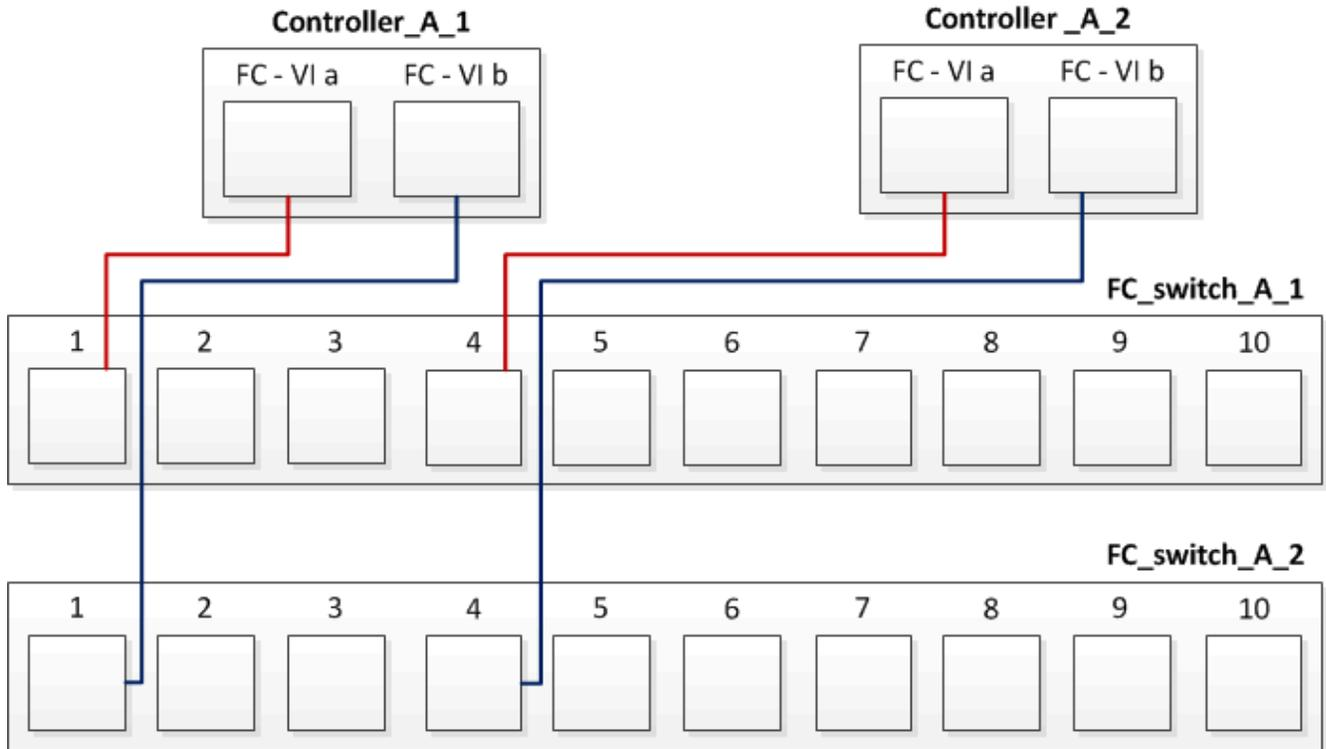
2. Perform the controller-to-switch cabling at both of the MetroCluster sites.
