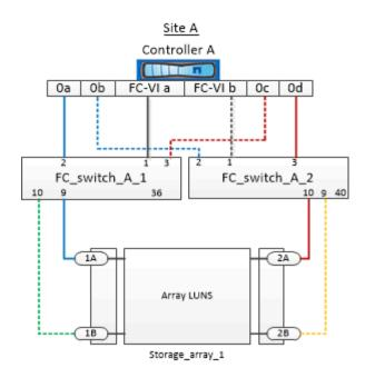
The connections between storage array ports and FC switch ports are similar for both stretch and fabric-attached variants of two-node MetroCluster configurations with array LUNs.
