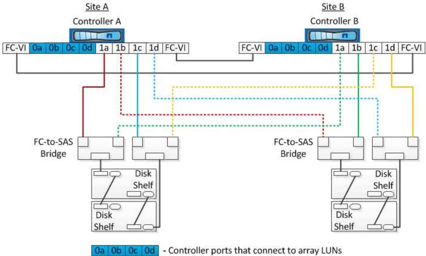
The following illustration shows a two-node stretch MetroCluster configuration with the array LUN connections:
