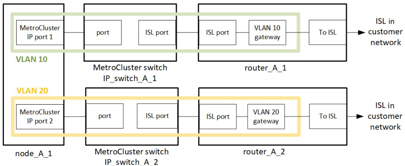
The MetroCluster environment is configured and cabled as a standard MetroCluster IP configuration as described in [Configure the MetroCluster hardware components](#). When you perform the installation and cabling procedure, you must perform the steps specific to a layer 3 configuration. The following applies to layer 3 configurations:
