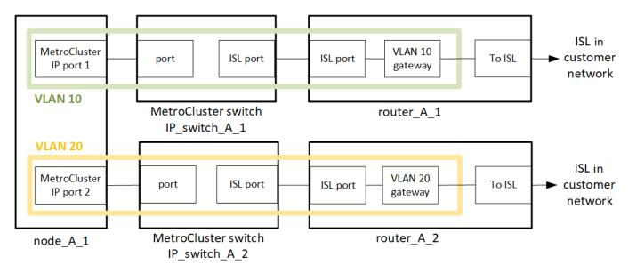
The MetroCluster environment is configured and cabled as a standard MetroCluster IP configuration as described in Configure the MetroCluster hardware components. When you perform the installation and cabling procedure, you must perform the steps specific to a layer 3 configuration. The following applies to layer 3 configurations:
