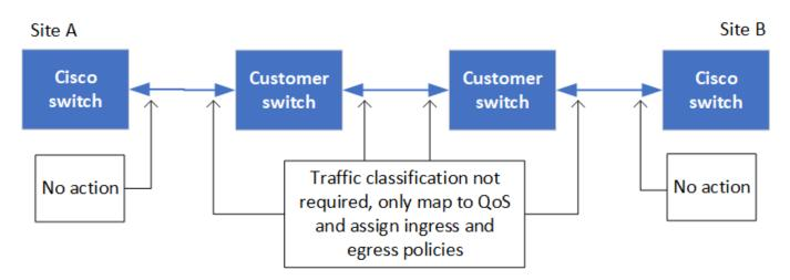
The following diagram gives an overview of the required settings for a shared network when the external switches are Broadcom IP switches.
