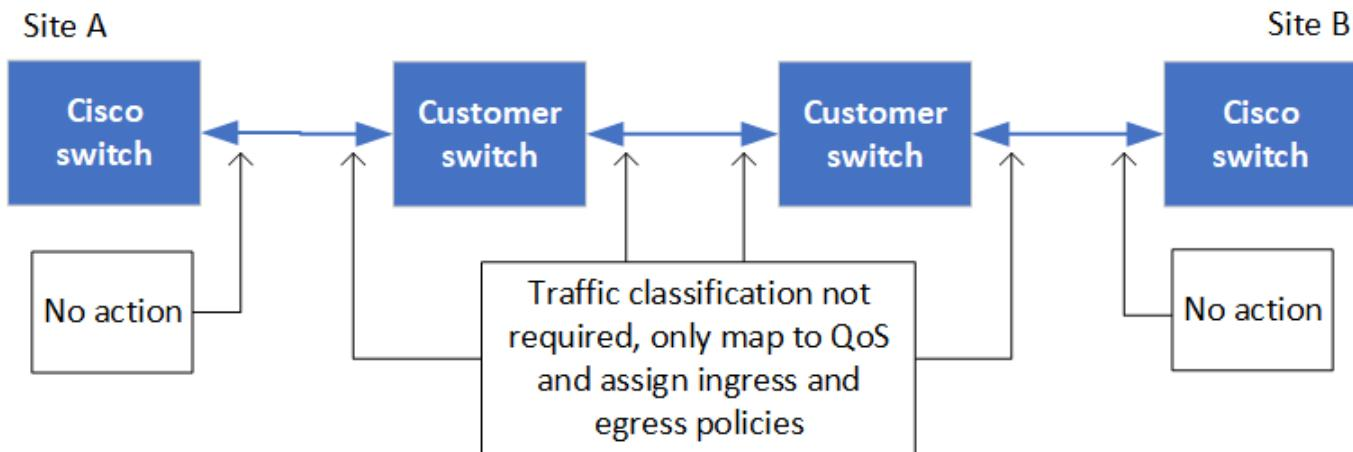
The following diagram gives an overview of the required settings for a shared network when the external switches are Broadcom IP switches.
