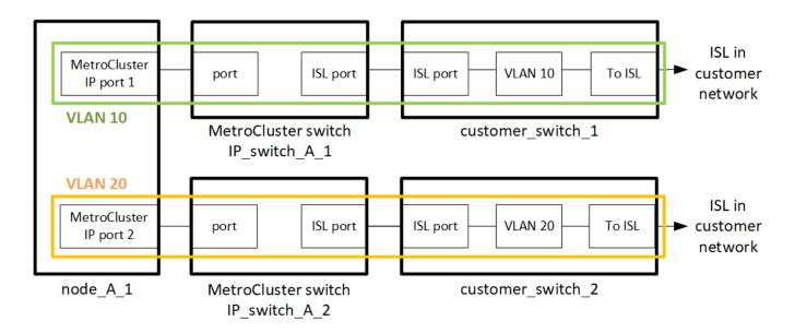
The intermediate customer-provided switches must meet the following requirements:
