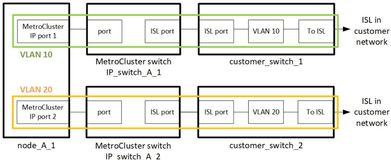
The intermediate customer-provided switches must meet the following requirements:
