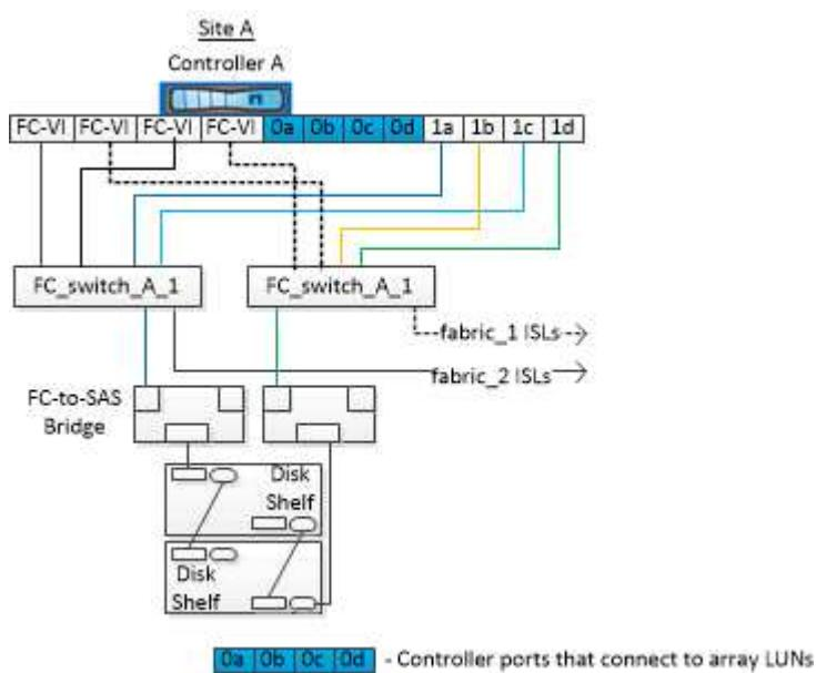
In the following illustration showing the connectivity between ONTAP systems and array LUNs, the HBA ports 0a through 0d are used for connectivity with array LUNs because ports 1a through 1d are used for connectivity with disks:
