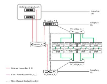
A two-node configuration includes the following connections:
