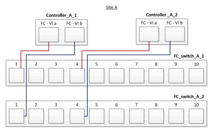
2. Perform the controller-to-switch cabling at both of the MetroCluster sites.
