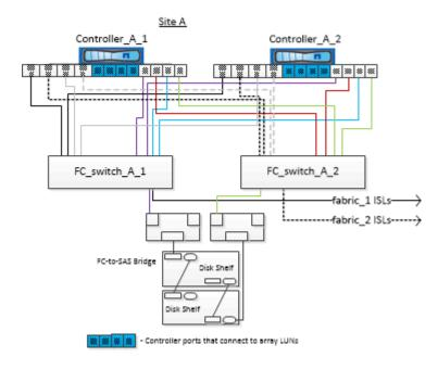
In the following illustration that shows the connectivity between ONTAP systems and array LUNs, the HBA ports 0a through 0d are used for connectivity with array LUNs because ports 1a through 1d are used for connectivity with disks:
