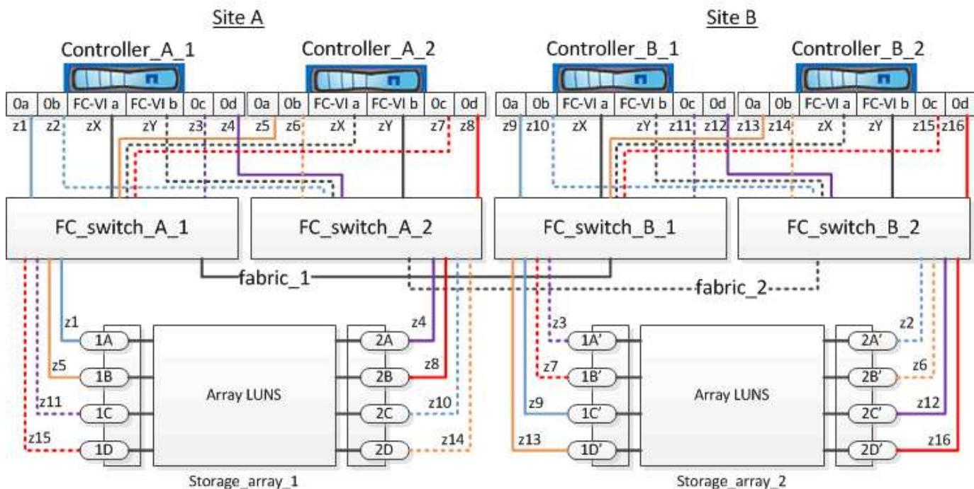
In the illustration, array LUNs are allocated on each storage array for the MetroCluster configuration. LUNs of equal size are provisioned on the storage arrays at both sites, which is a SyncMirror requirement. Each ONTAP system has two paths to array LUNs. The ports on the storage array are redundant.
