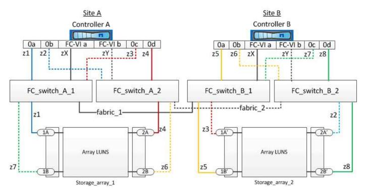
The example shows single-initiator to single-target zoning for the MetroCluster configurations. The lines in the example represent zones rather than connections; each line is labeled with its zone number.
